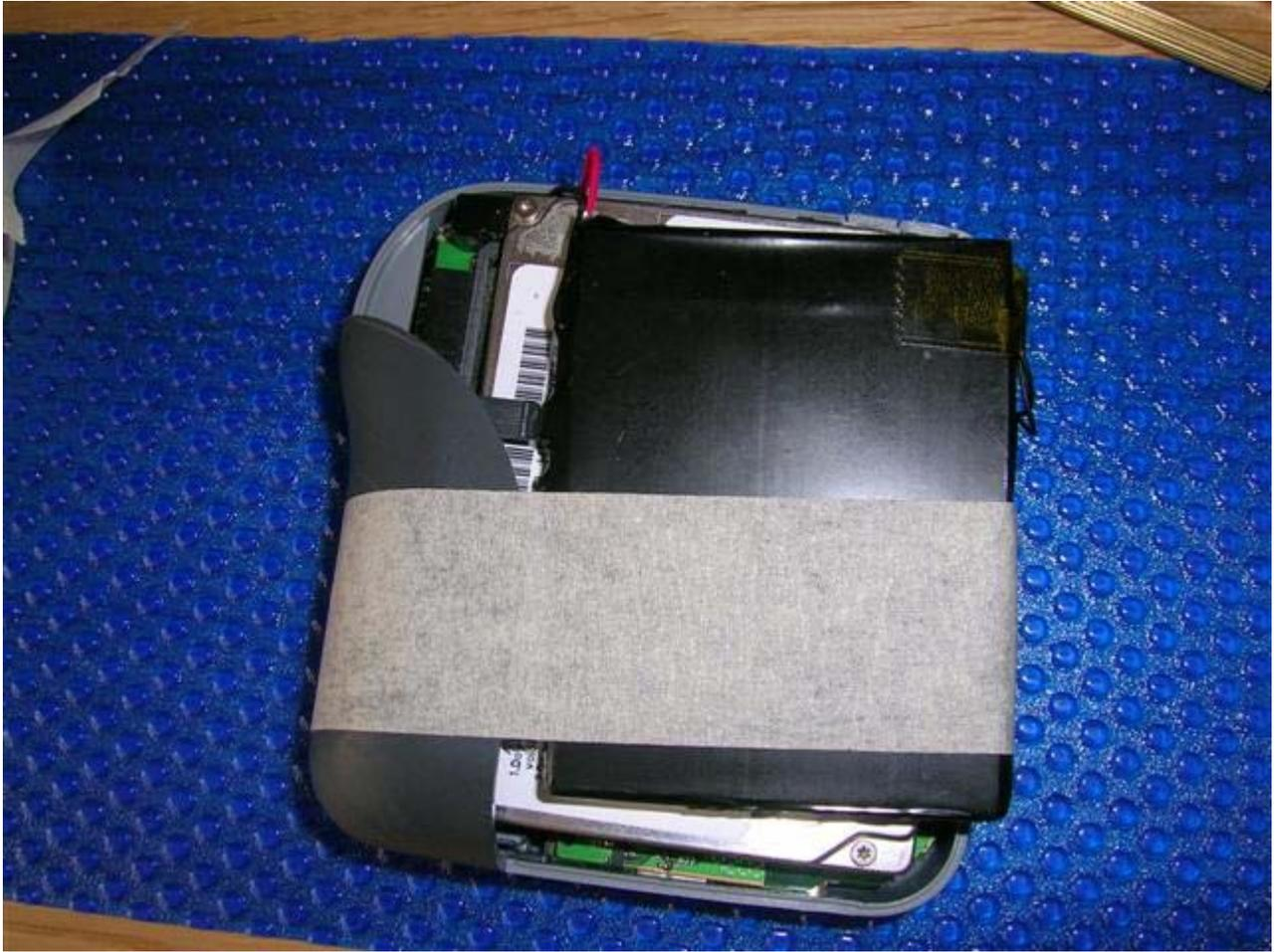
Once it's all back together, it's a good idea to let the player fully charge, there have been occasions where it might not switch on due to the battery being discharged after removal. Or if you're impatient like me just power it up and then plug into the USB dock and flash with the latest firmware (I used Rio's own flash tool).
