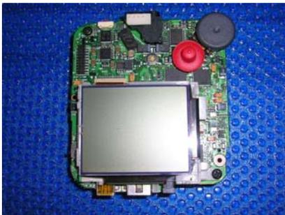
Once the front is off, carefully bend the back cover slightly so it peels off.
