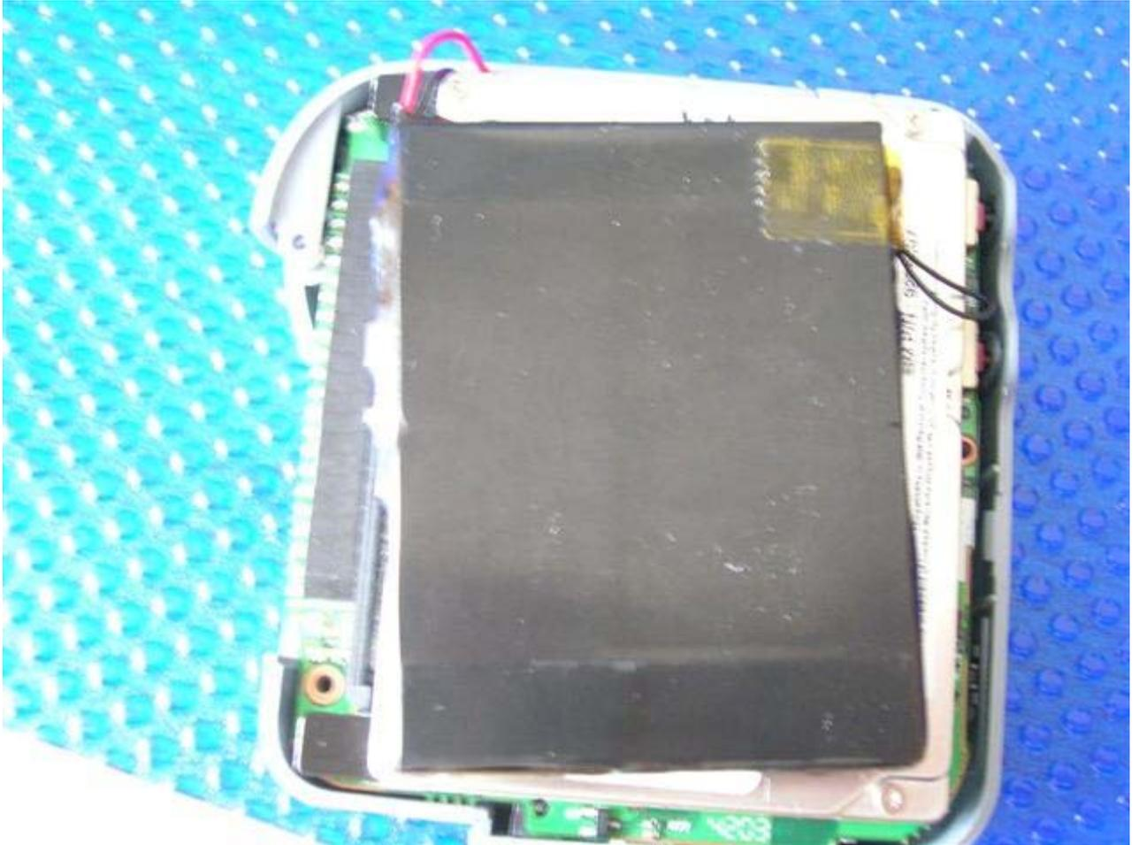
Now unclip the battery and the power circuit from the main board and set it aside.
