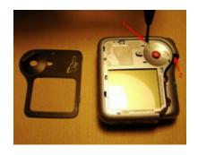
7. With the lens and side panel off, you will see two screws now exposed. Remove these two screws.
