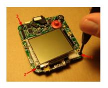
17. With the LCD now loose on its ribbon cable, you can access all three of the screws holding the hardrive. Remove them.
