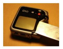
5. Starting at the bottom right corner, slide your putty knife under the lens and gently twist to separate it from the case. Be careful not to insert the putty knife so far as to overlap the LCD screen and potentially damage it. The lens is held down with double sided tape, and is relatively easy to pry up.
