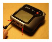
3. Using your Phillips screwdriver, remove the two screws on the bottom of the player.
