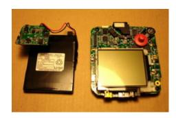
15. With the battery circuit board disconnected, the battery is free.
