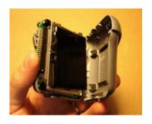
9. The back case piece should now come off easily, starting from the scroll wheel side and hinging open like a pizza box.
