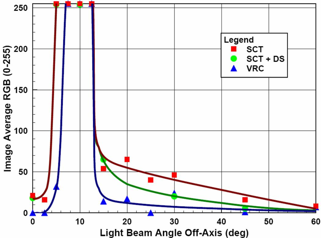
Figure 38 Test #7 – Measured Off-Axis Light Rejection
