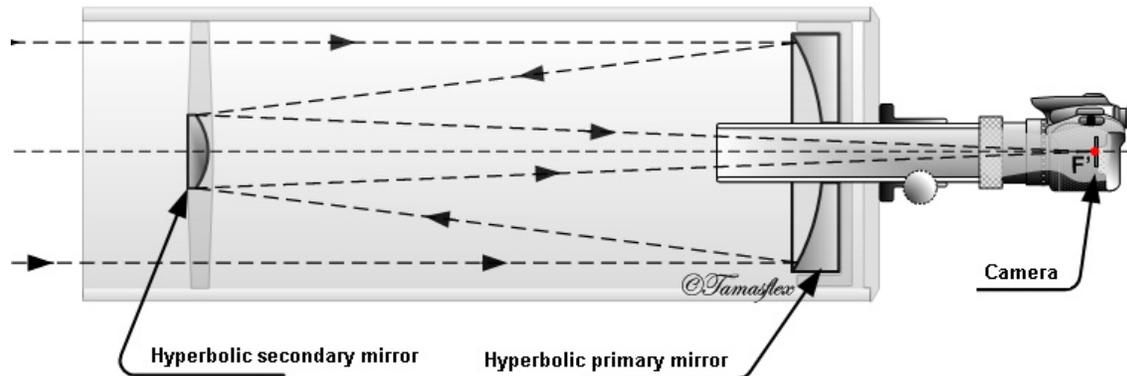
Figure 2 Schematic of a Ritchey-Chretien Telescope
