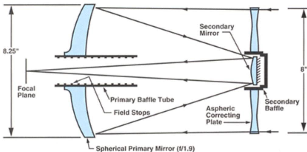
Figure 1 Schematic of a Schmidt-Cassegrain Telescope (Meade 8")
