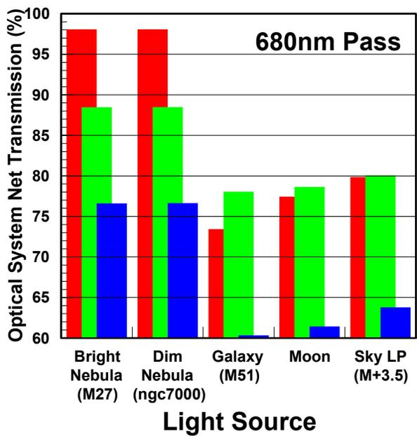
Figure A-3 Predicted Optical System Net Transmission – Mallincam Use
