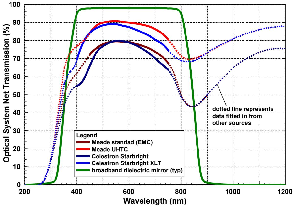
Figure A-1 Optical System Spectral Transmission By Coating System
