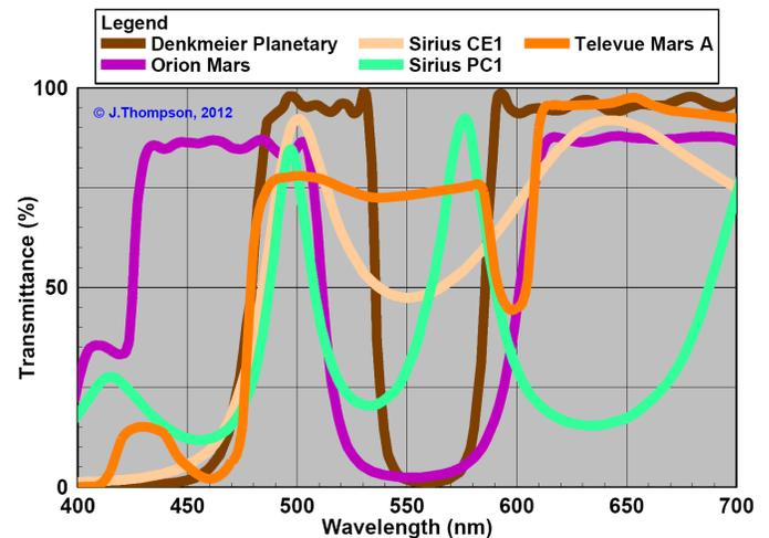
**Figure 2. Spectral Response of Special Planetary Filters:** Interference coating technology has been used to make filters that improve the contrast of planetary surface features.
