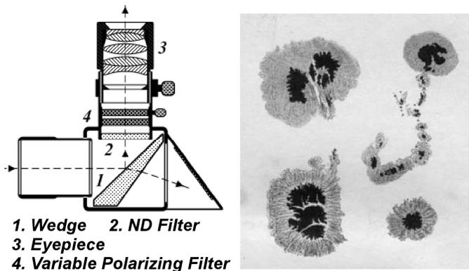
**Figure 5. The Herschel Wedge:** John Herschel first proposed the idea of using a wedge to split off a safe amount of sunlight for observation (left). His resulting observation sketches are as impressive today as they were 150 years ago (right).
