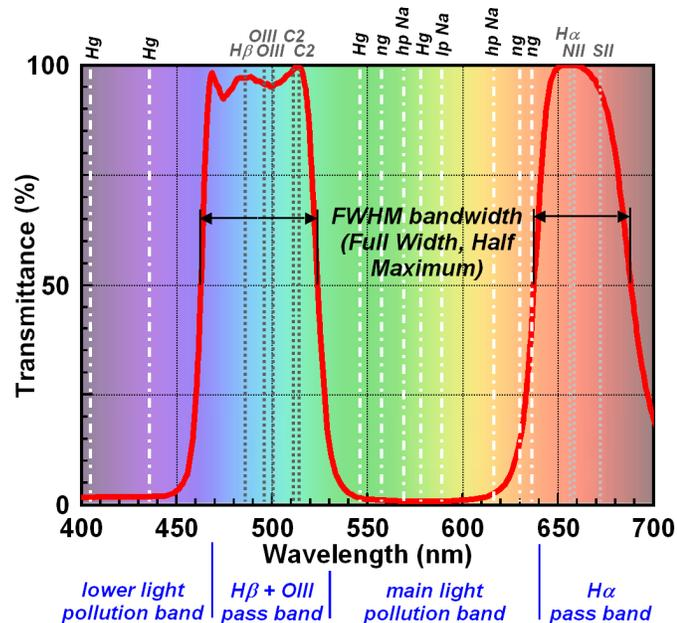
**Figure 2. Example Spectral Transmissivity Plot:** Deep-sky filters tend to have similar appearance as they are trying to achieve the same goal, pass the desirable H $\beta$ +OIII & H $\alpha$  passbands, and cut the undesirable light pollution bands. Note that “bandwidth” is normally defined at half the maximum transmittance value of the filter, known as FWHM.
