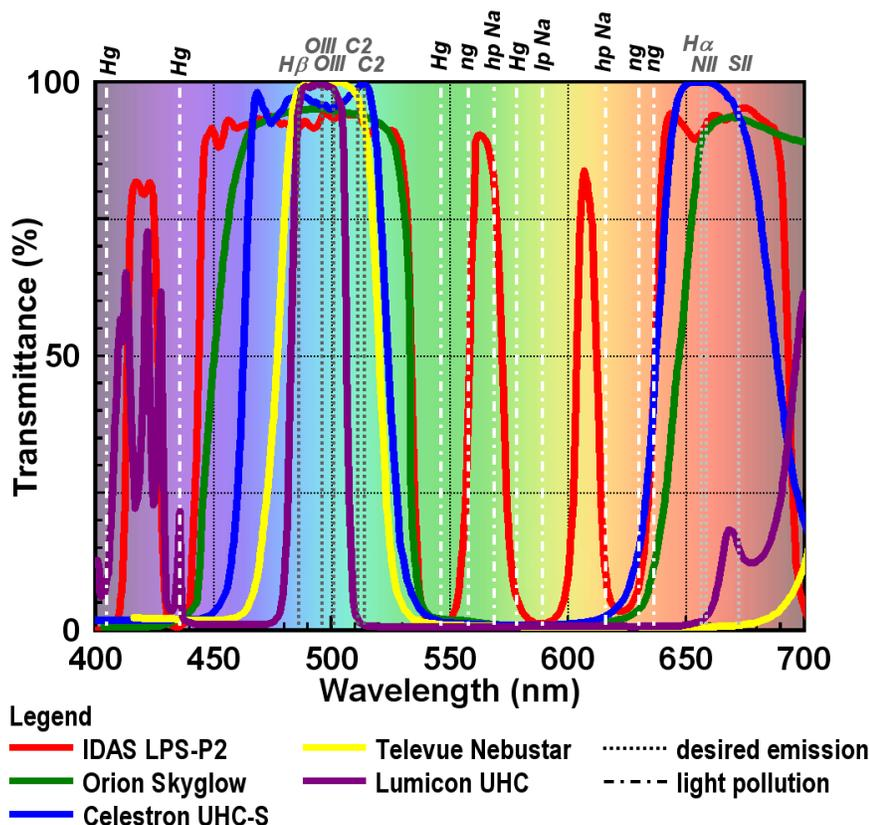
**Figure 5. Example Data Available From Manufacturers:** Most manufacturers of deep-sky filters provide spectral transmissivity data for their products, however the buyer needs more information to make a properly informed purchase.
