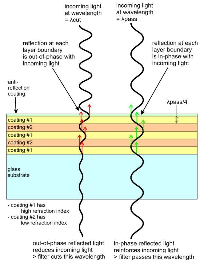
**Figure 3. How Interference Filters Work:** At each interface between filter layers, some light is reflected. The reflected light interacts with the incoming light, attenuating some wavelengths and amplifying others as defined by the layer thicknesses.
