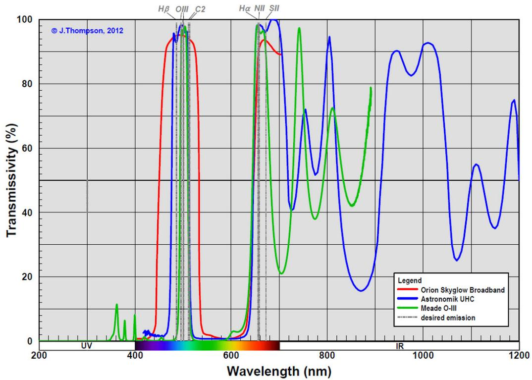
Figure 2 Spectral Response Curves - LP Filters
