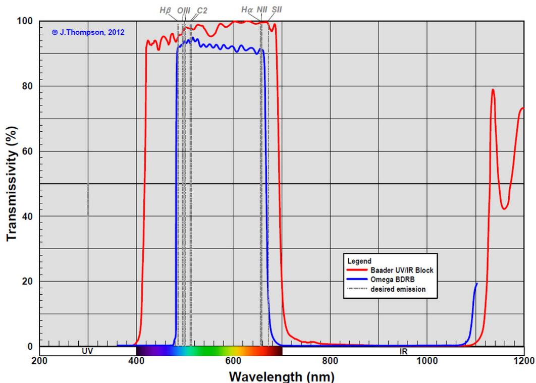
Figure 1 Spectral Response Curves - UV/IR Blocker Filters
