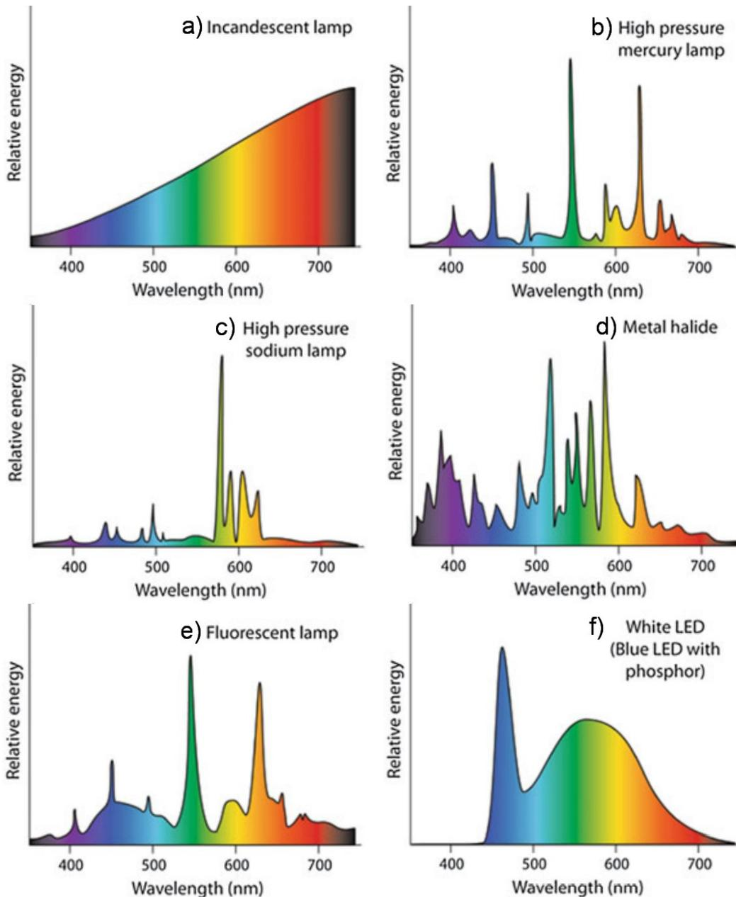
Figure 1 Typical Spectra for Different Man-Made Lighting Technologies<sup>1</sup>
