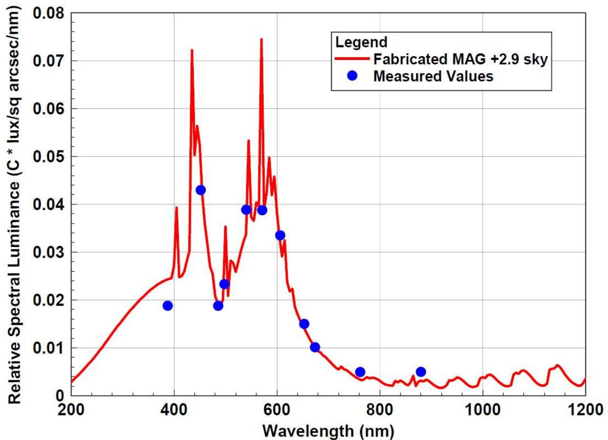
Figure 6 Measured Backyard LP Spectrum vs Fabricated
