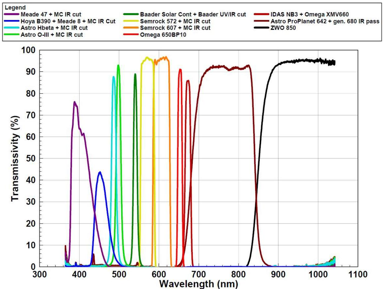
Figure 5 Measured Spectra for Selected Filter Combinations
