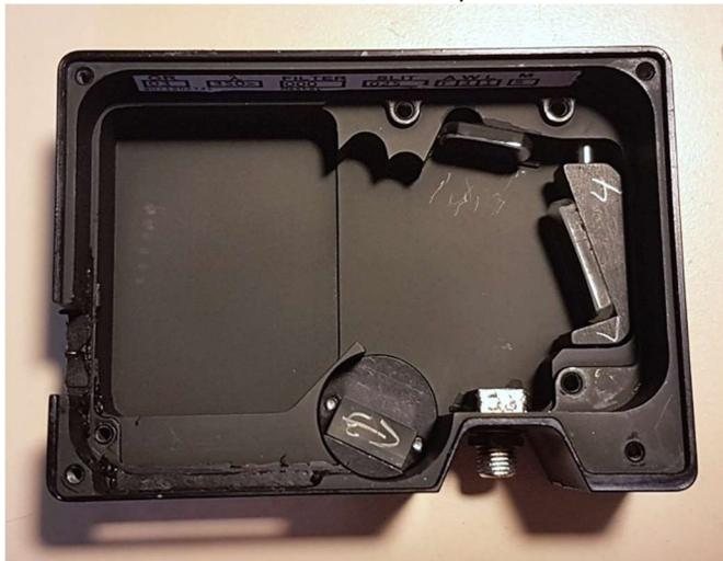
*Circuit board removed, exposing optical bench*
