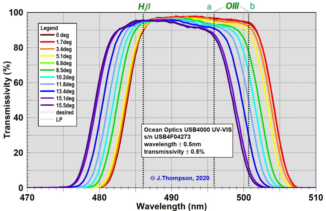
Figure 4 Measured Radian Triad Spectral Response vs Angle – O-III Pass Band
