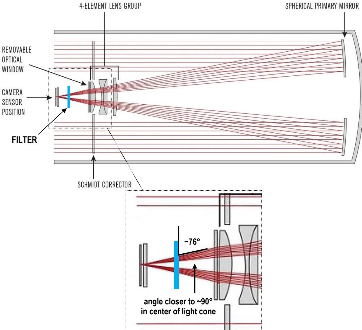
Figure 12 Schematic of Light Path Inside Celestron RASA Telescope (courtesy Celestron)
