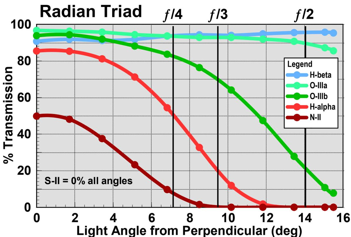
Figure 9 Measured Radian Triad Nebula Wavelength Transmission vs Angle
