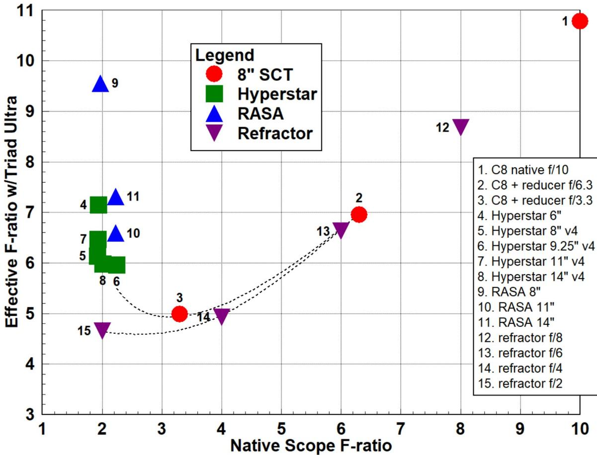
Figure 14 Prediction of Triad Ultra Filter Impact on Scope Effective F-ratio – H-alpha Band
