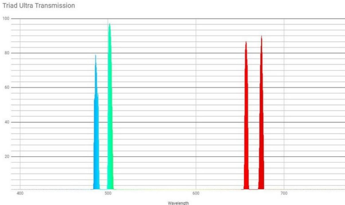
Figure 2 OPT Radian Triad Ultra Spectral Response (courtesy OPTCorp)
