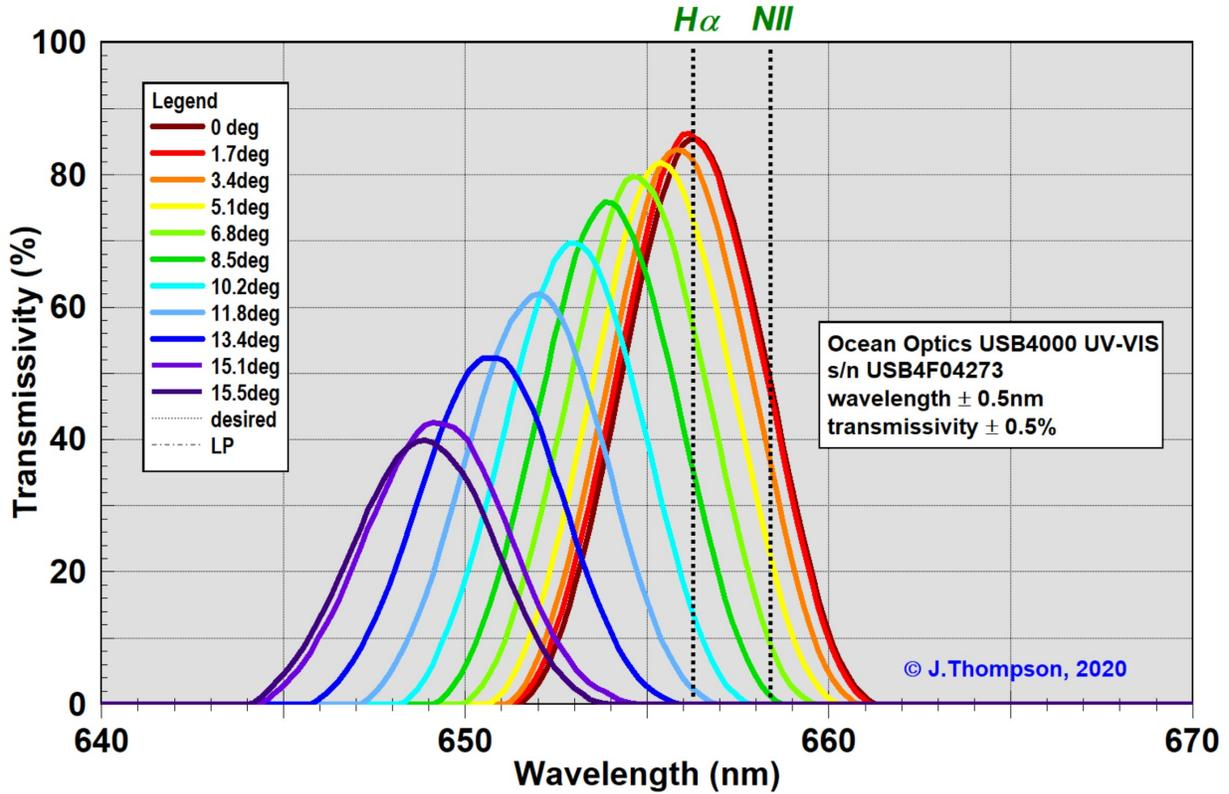
Figure 5 Measured Radian Triad Spectral Response vs Angle – Halpha Pass Band
