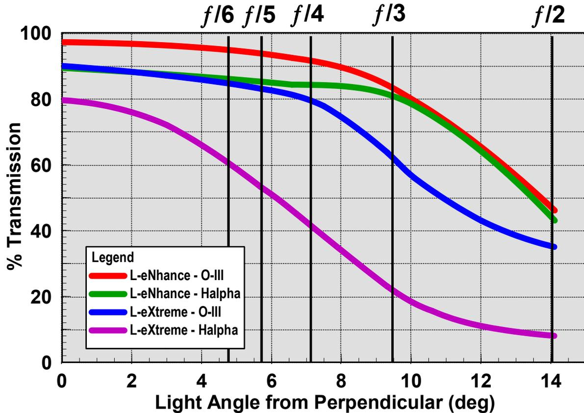
Figure 12 Impact of Angle On Filter Performance
