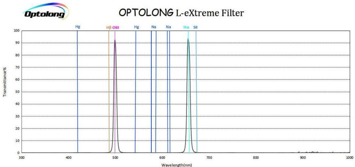
Figure 1 Spectral Response of the New L-eXtreme Filter
