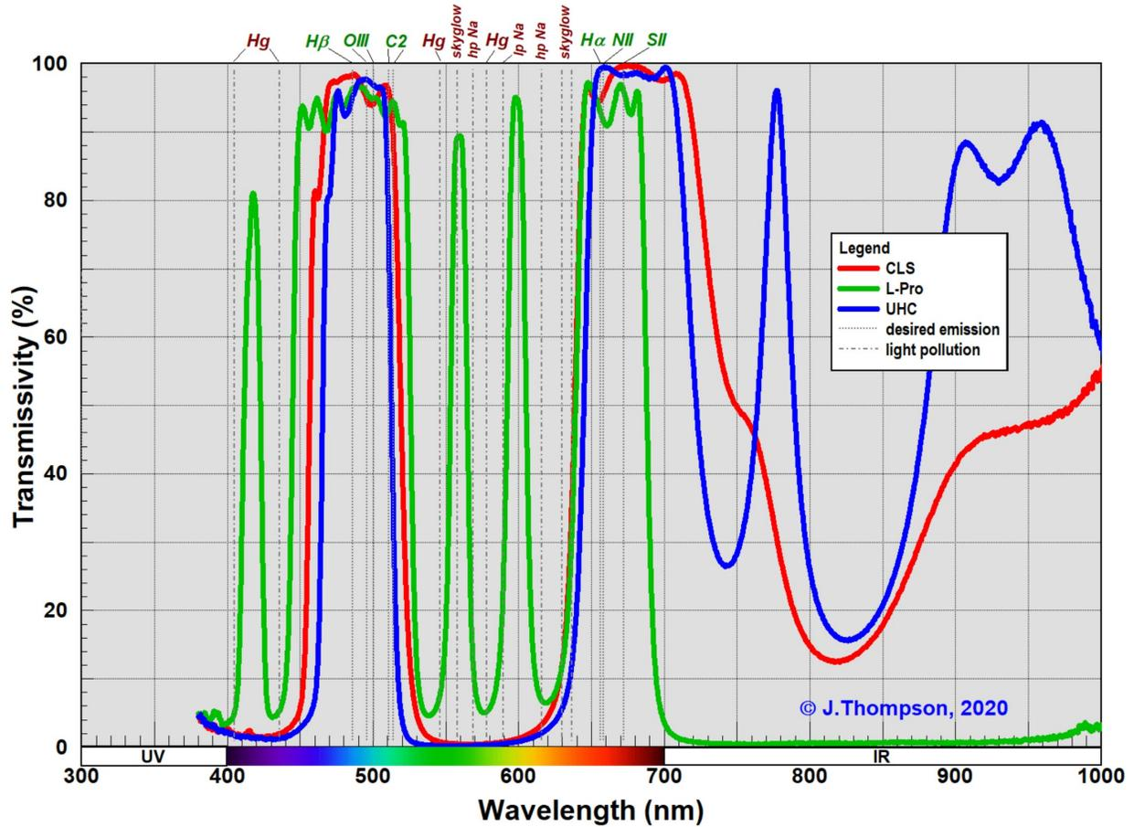
Figure 2 Measured Spectral Response of Optolong Filters – 1
