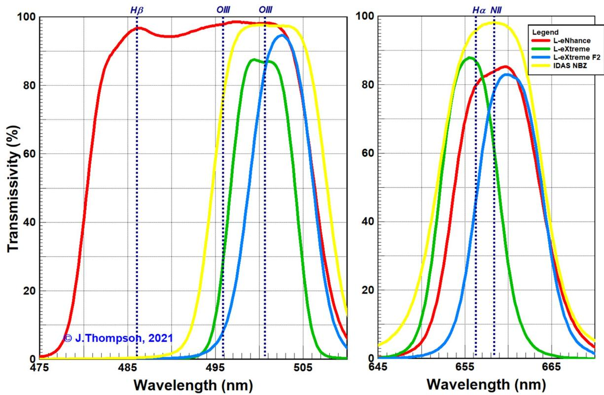
Figure 4 Net Spectral Response of Tested Filters – f/6.3 Refractor Area Weighted Average
