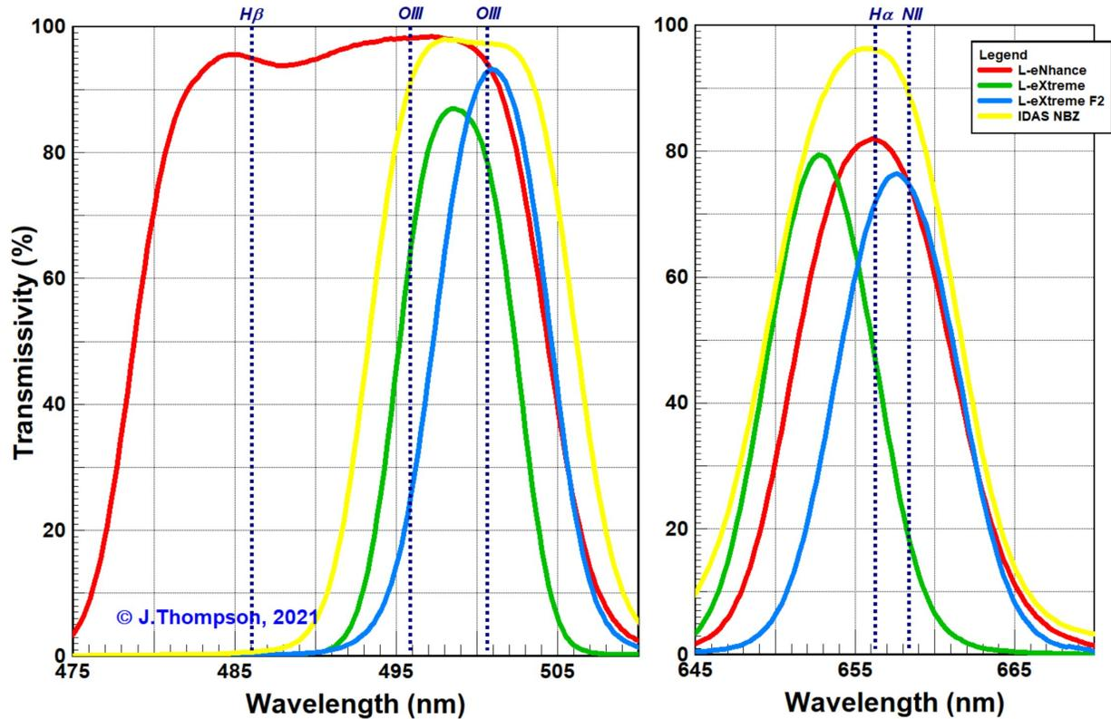
Figure 5 Net Spectral Response of Tested Filters – f/2 C14 w/Hyperstar Area Weighted Average
