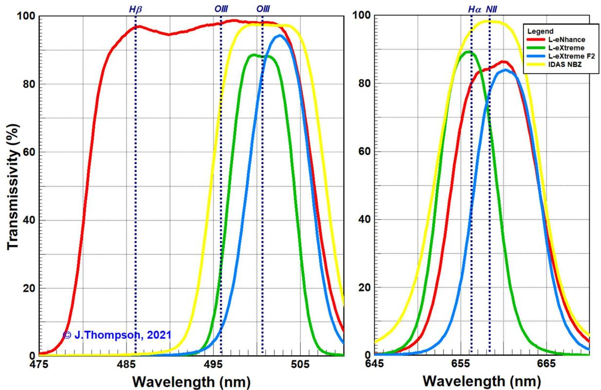
Figure 1 Measured Spectral Response of Tested Filters – Filter Perpendicular to Light Path
