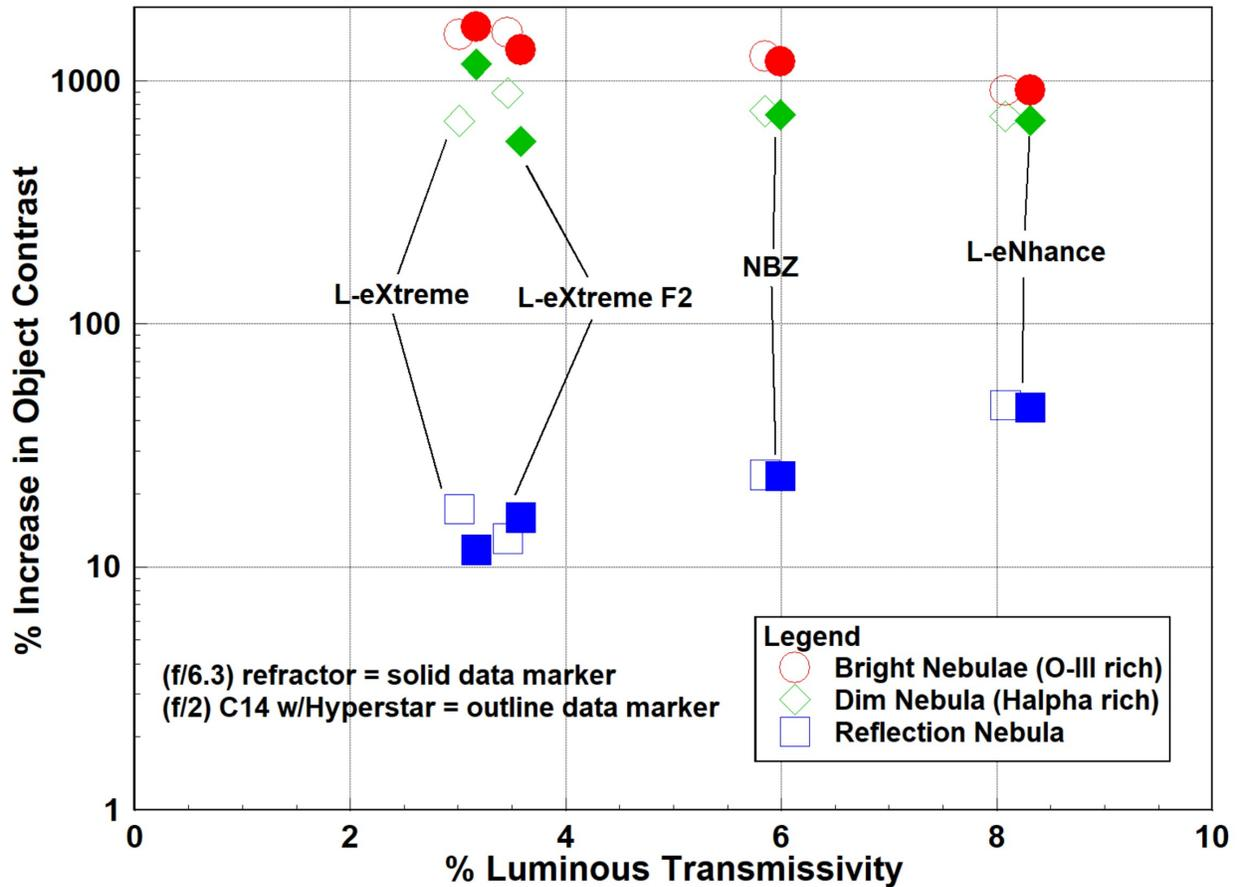
Figure 6 Predicted Filter Performance: Back Illuminated Colour CMOS, LP w/LED (NELM+2.9)
