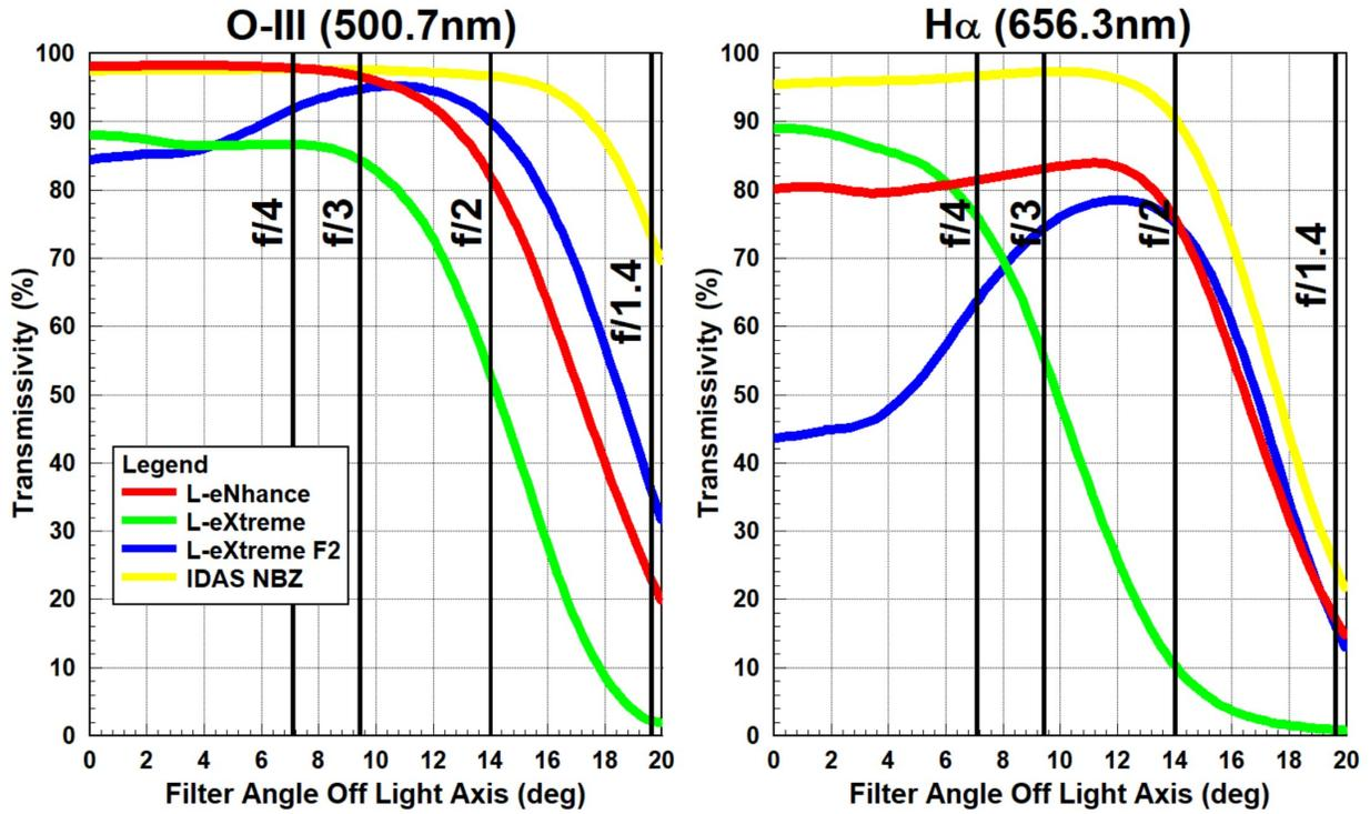
Figure 2 Measured Impact of Angle on Filter Response
