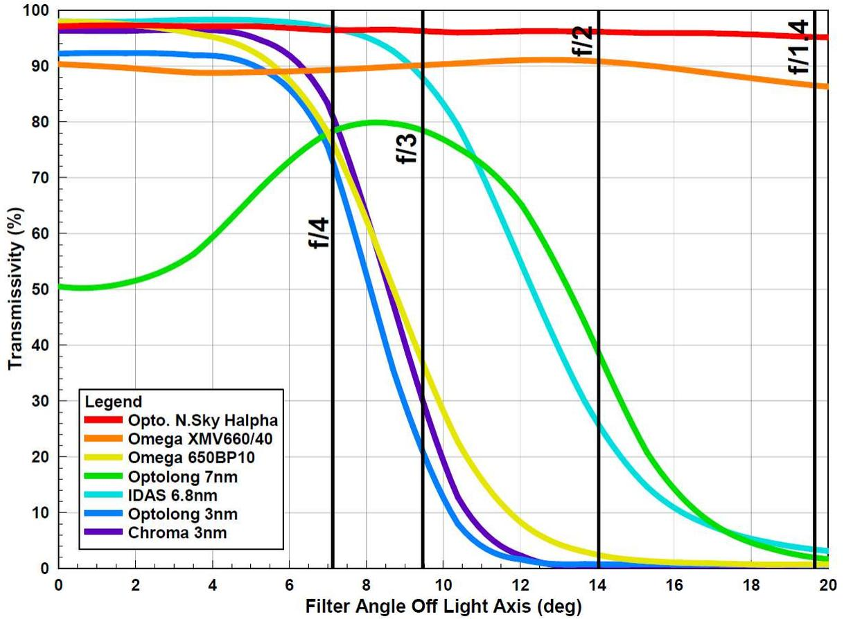
Figure 2 Measured Impact of Angle on Filter Response
