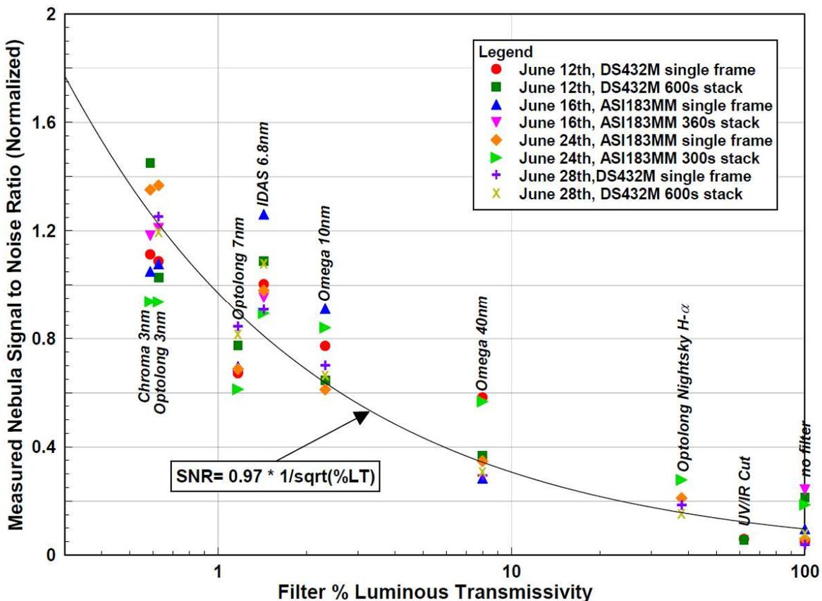
Figure 15 Measured Nebula Signal-to-Noise Ratio
