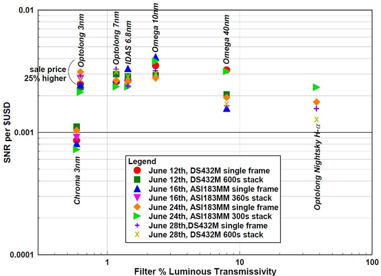
Figure 16 Filter Signal-to-Noise Ratio per \$USD
