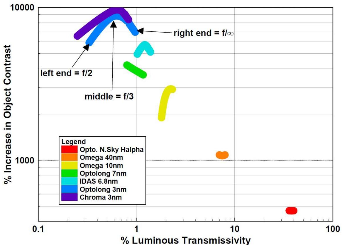
Figure 8 Predicted Filter Performance: Back Illuminated Monochrome CMOS, LP w/LED (NELM+2.9)
