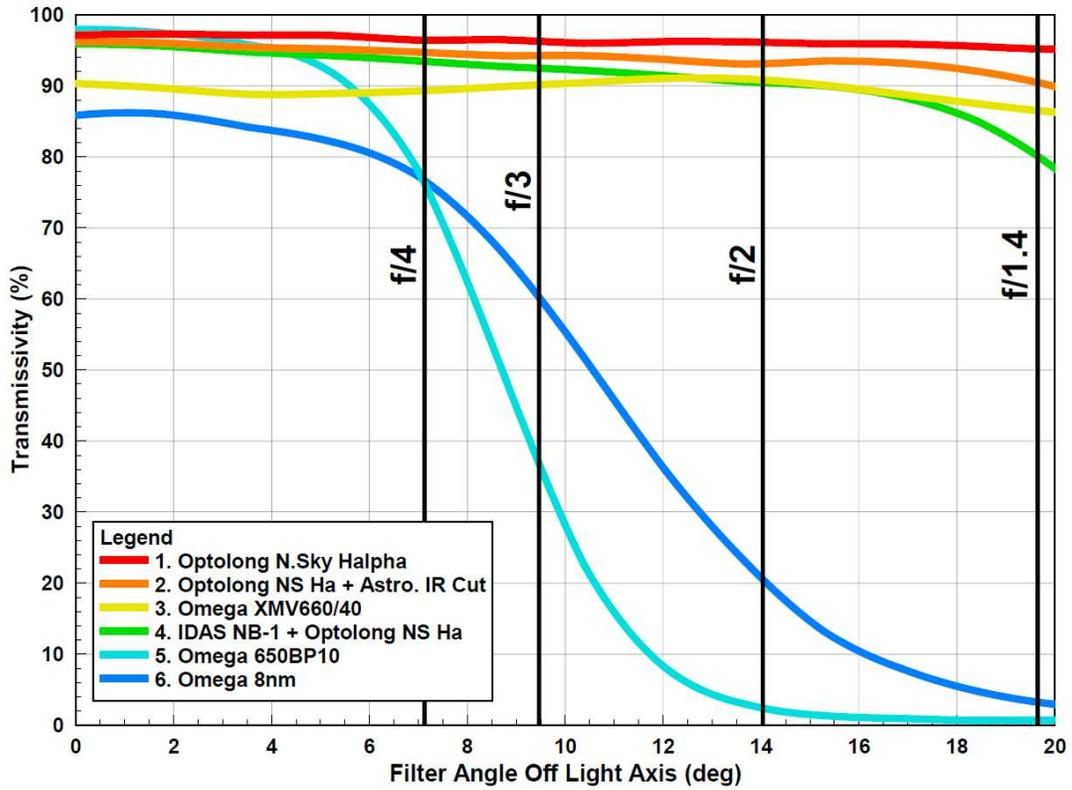
Figure 5 Measured Impact of Angle on Filter Response, FWHM >8nm
