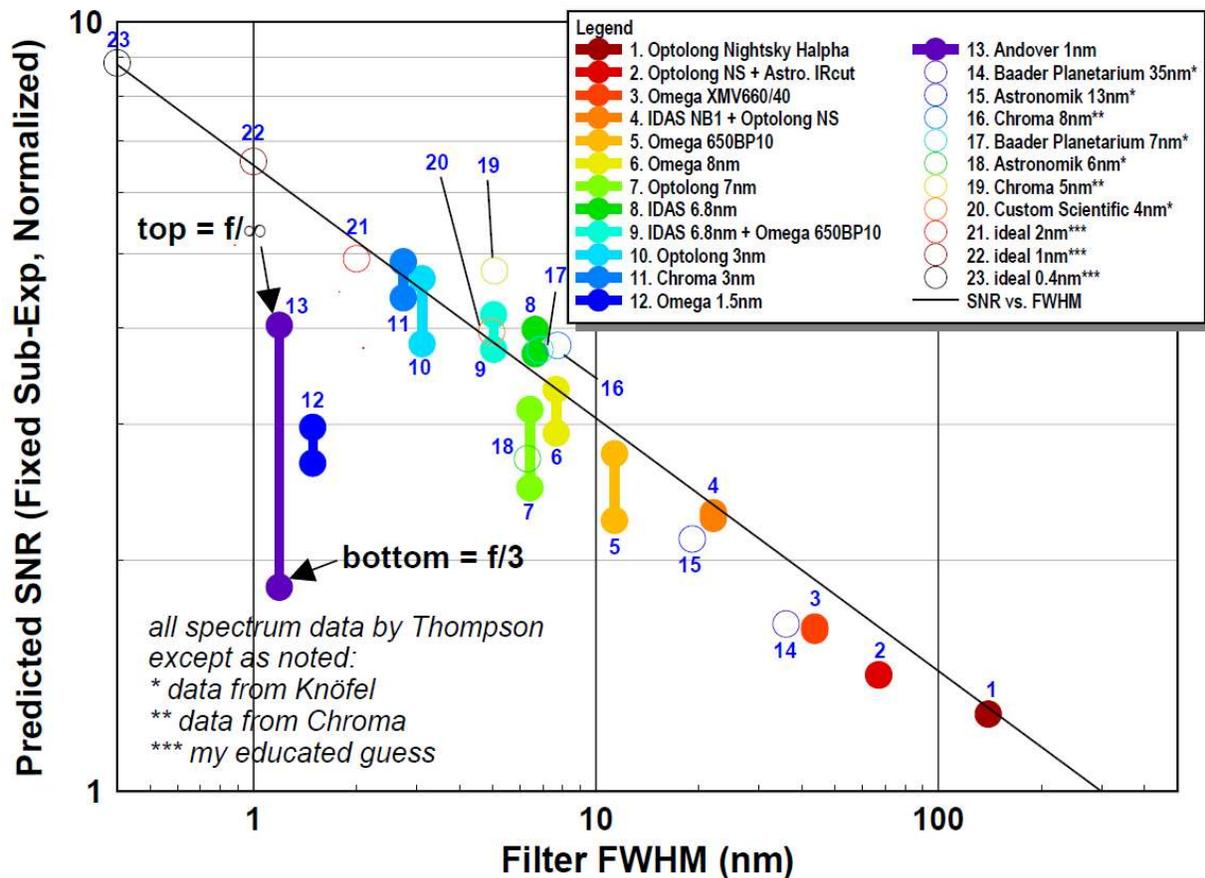
Figure 9 Predicted SNR: Back Illuminated Monochrome CMOS, LP w/LED (NELM+2.9)
