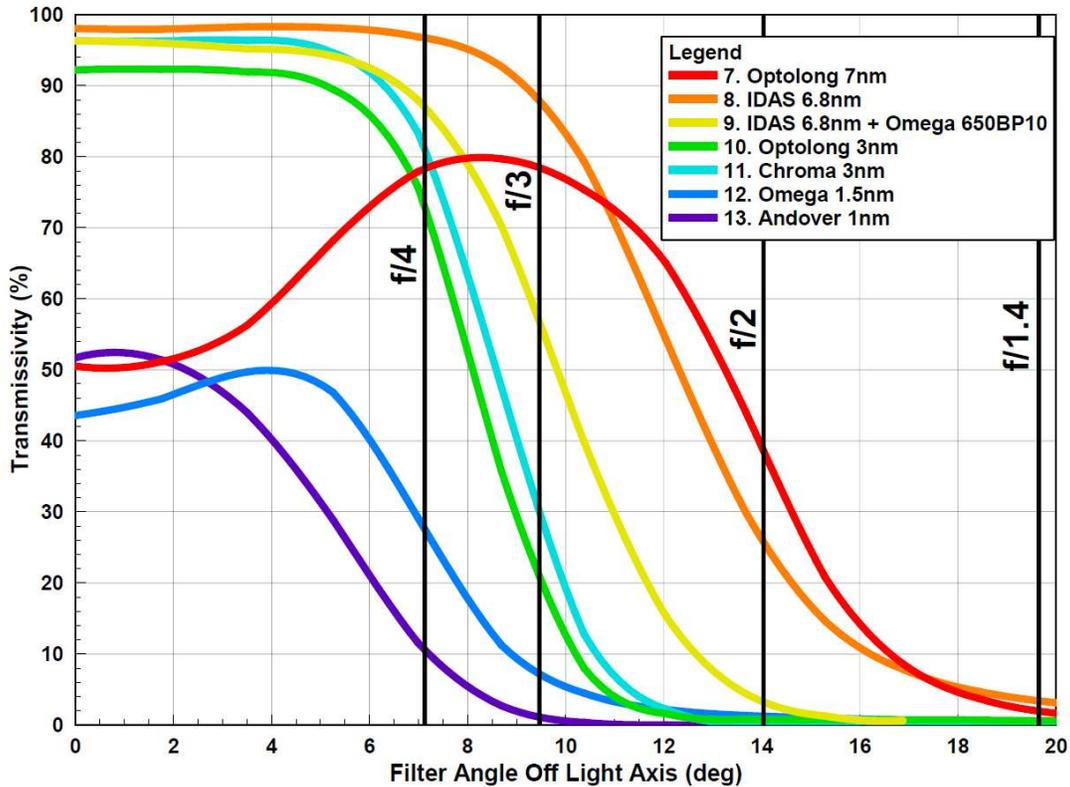
Figure 6 Measured Impact of Angle on Filter Response, FWHM <8nm
