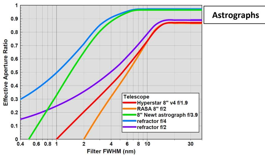
Figure 7 Predicted Effect of Filter Band Shift in Terms of Effective Aperture for Various Scope Types
