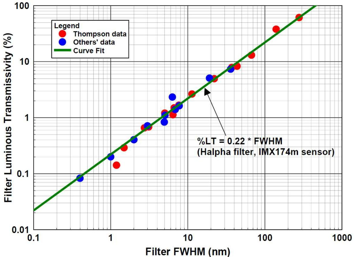
Figure 10 Calculated %LT vs FWHM for Tested Filters
