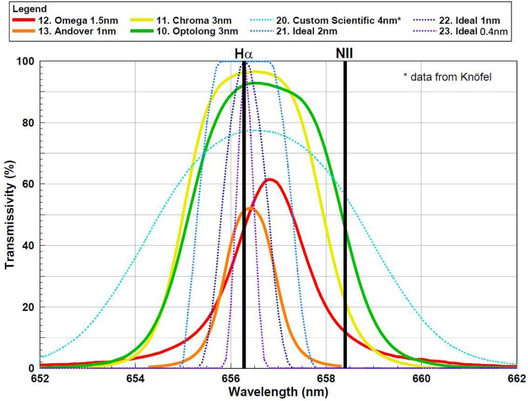
Figure 4 Measured Filter Spectra – Filter Perpendicular to Light Path, FWHM <5nm
