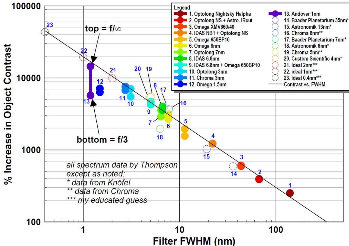
Figure 8 Predicted Contrast Increase: Back Illuminated Monochrome CMOS, LP w/LED (NELM+2.9)
