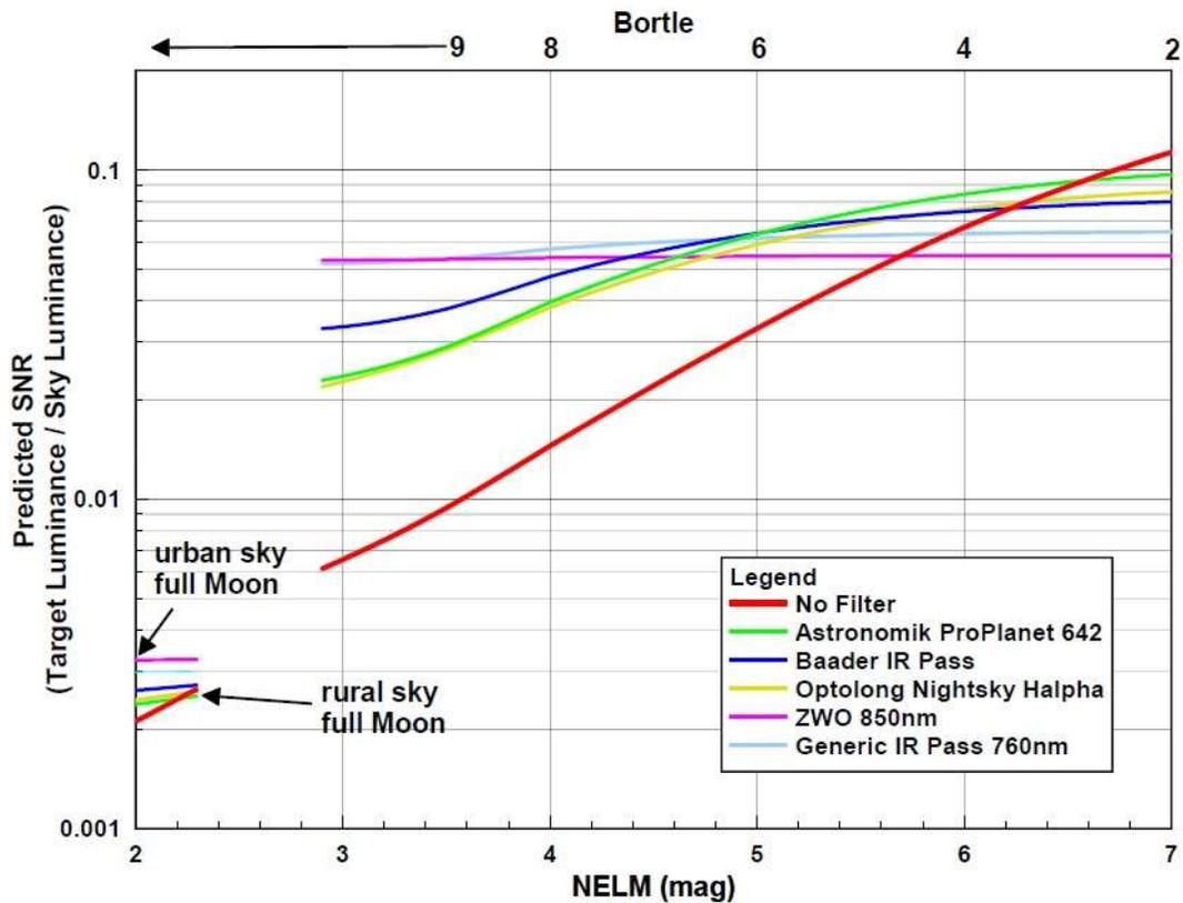
Figure 10 Predicted Filter Performance For Varying Sky Darkness – IR Pass
