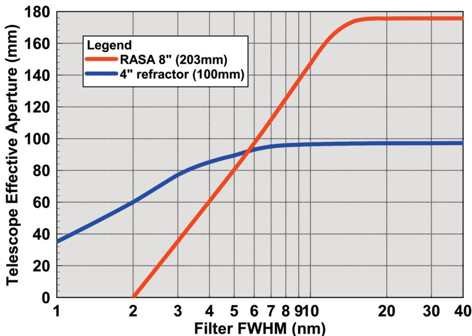
Figure 5 - Predicted Scope Effective Aperture vs Filter FWHM
