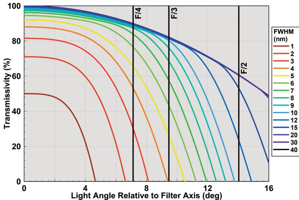
Figure 4 - Predicted Generic Filter H-alpha Transmission vs Angle
