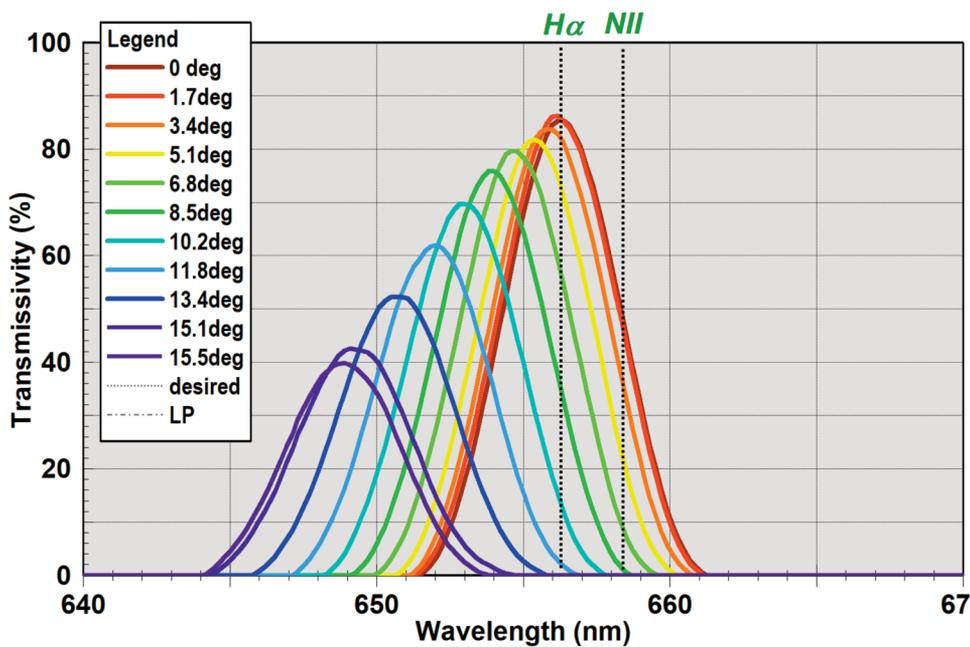
Figure 2 - Measured Spectral Response of Radian Triad Filter vs Angle – H-alpha Band
