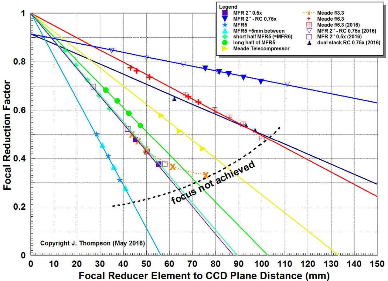
Figure 4 Focal Reduction Factor vs. FR-to-CCD Plane Distance
