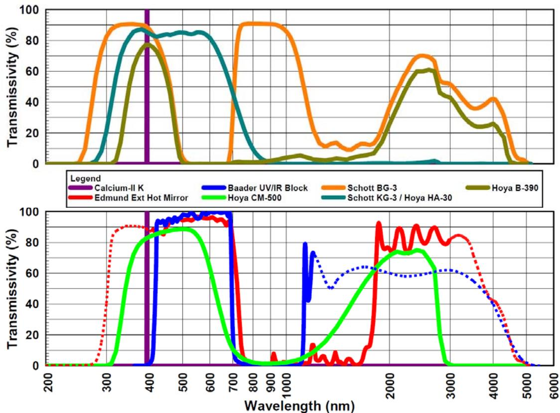
Figure 5: Response curves for the filters used in solar heating tests. (graphs by J. Thompson)
