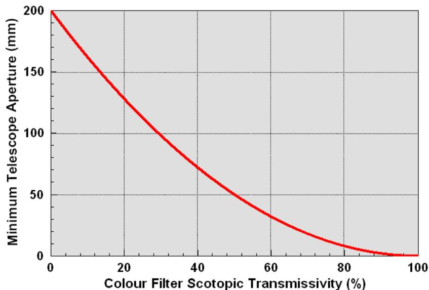
**Figure 9 Minimum Recommended Aperture Size for Colour Filters**
