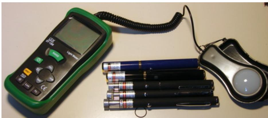
**Figure 6 Main Components of My Make-Shift Spectrum Analyser**
