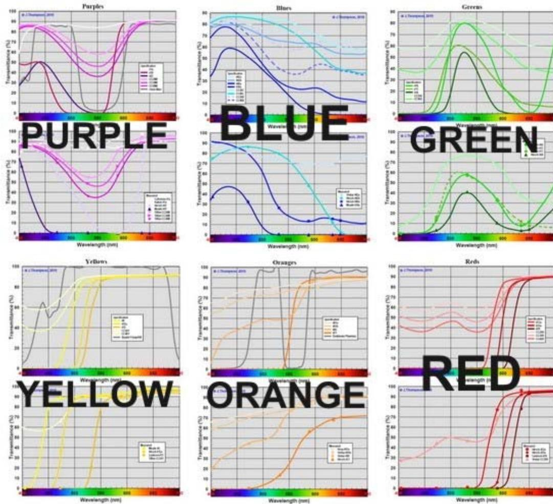
Figure 8 Colour Filter Spectral Response Curves
