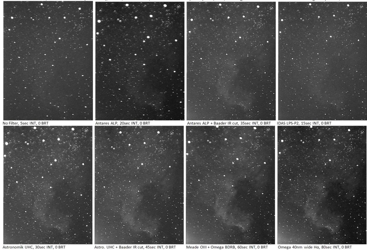
**Figure 1** Screen Captures from 1<sup>st</sup> Experiment w/ LP Filters + Monochrome Cameras
