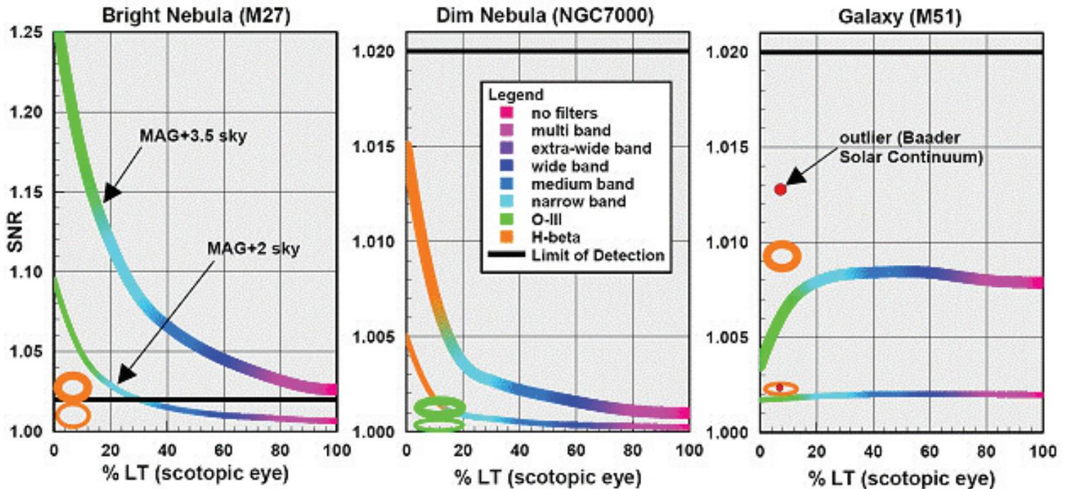
Figure 7. All Deep-Sky Filters Compared: These plots are a simplified view of predicted performance for all interference-type filters for which I have data.
