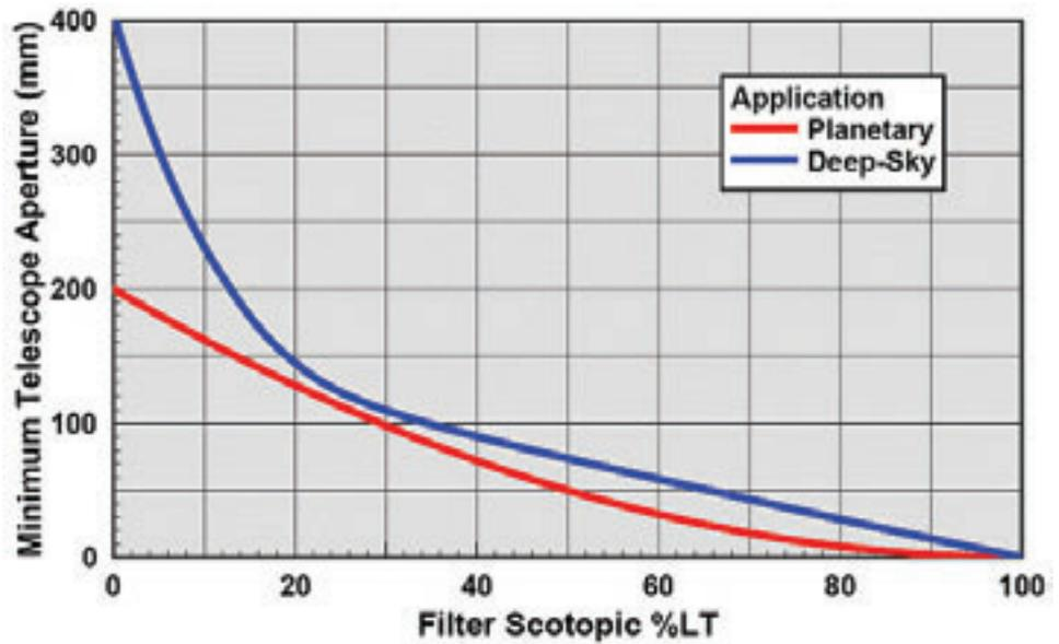
Figure 6. Recommended Minimum Percentage LT Versus Aperture: All filters reduce the amount of light getting to the eye. It is important to pick a filter that is not too dark for your aperture.
