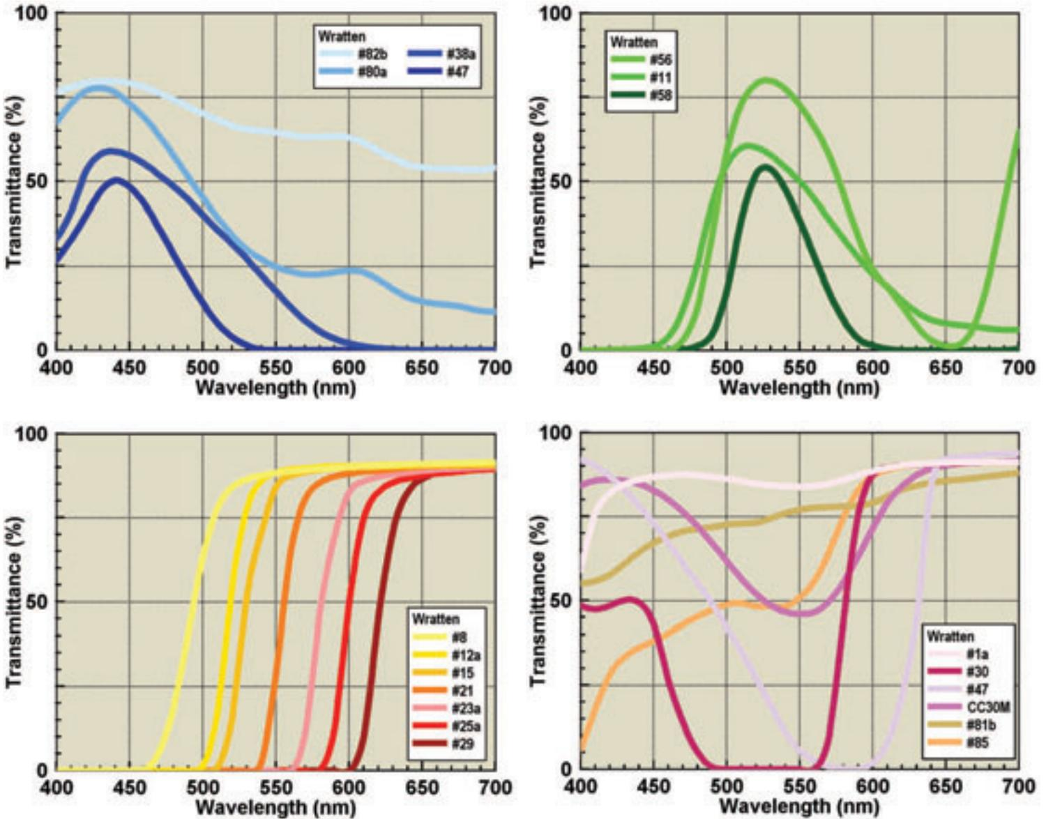
**Figure 3. Spectral Transmissivity of Planetary Filters:** Colour filters for astronomy can be grouped based on their general spectral response shape: blues, greens, and yellow-reds. Some additional Wratten filters are worth trying if available such as the violet-magentas and orange-browns.
