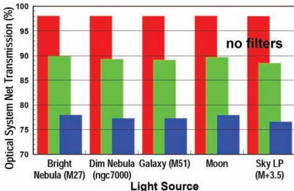
**Figure 2: Predicted Optical System Net Transmission – Visual Use: The improvement in image brightness between standard coatings, UHTC coatings, and dielectric coatings is consistent regardless of the target when the scopes are being used visually.**
