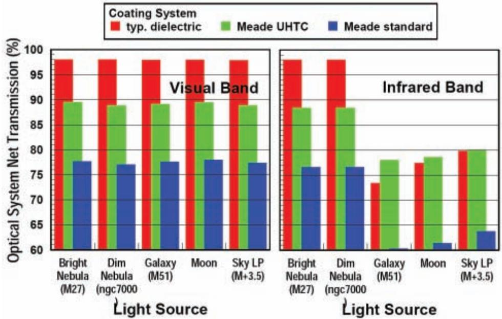
**Figure 3: Predicted Optical System Net Transmission – CCD Use: In the visual band, the difference in image brightness between different coatings is very similar with a CCD as it is for visual observation. The performance is quite different in the near-infrared band however, having implications when viewing IR-rich objects like galaxies, globular clusters, the Moon or even planetary work.**
