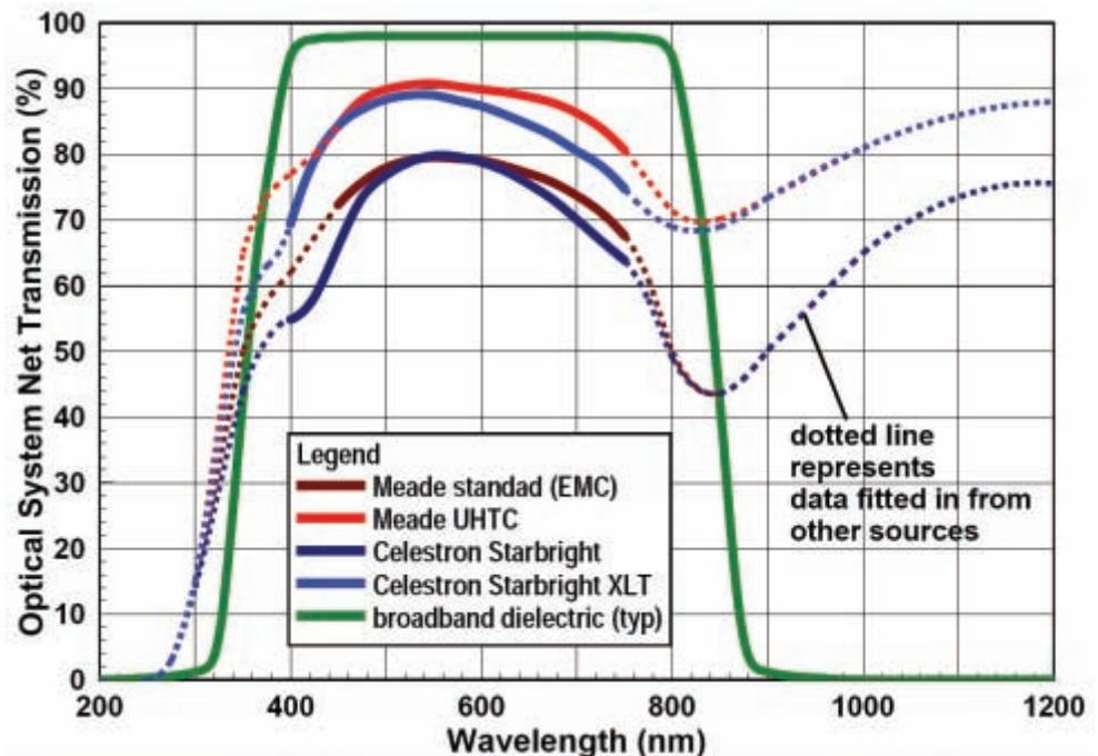
Figure 1: Optical System Spectral Transmission By Coating System: Total system response data is available from Meade and Celestron for the visual band. Data for outside the visual band, and for a typical dielectric mirror has been estimated by combining data from several third-party sources.
