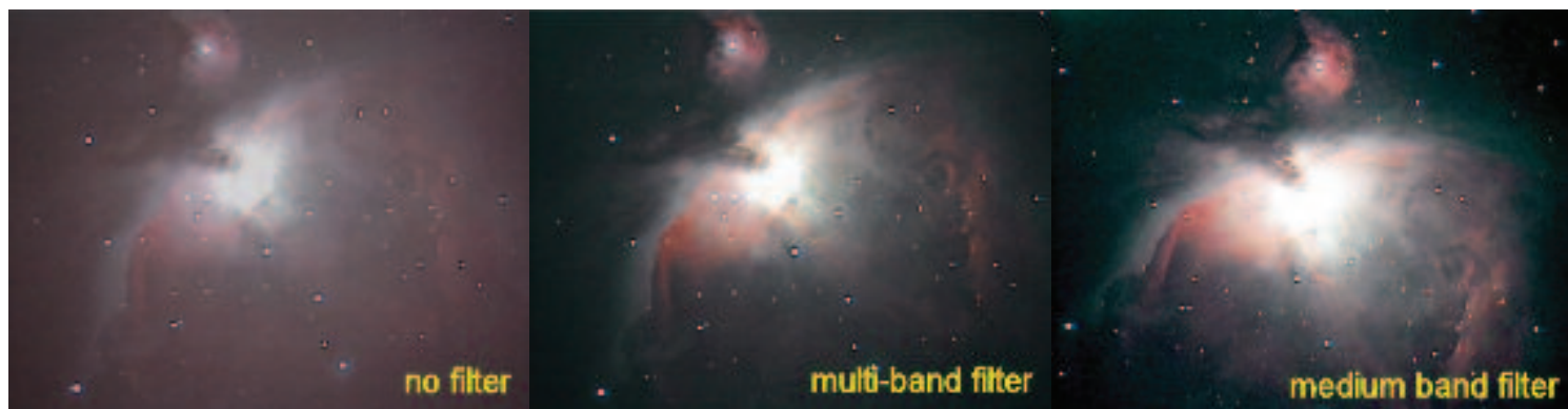
Figure 4. Effect of Deep-Sky Filters On M42: These images illustrate the impact of a range of different categories of deep-sky filter on the emission nebula M42. As the width of the band pass becomes narrower and narrower, more light pollution is filtered out, and the contrast between background and nebula is increased. In addition, star brightness is reduced, further increasing contrast in the nebula.
