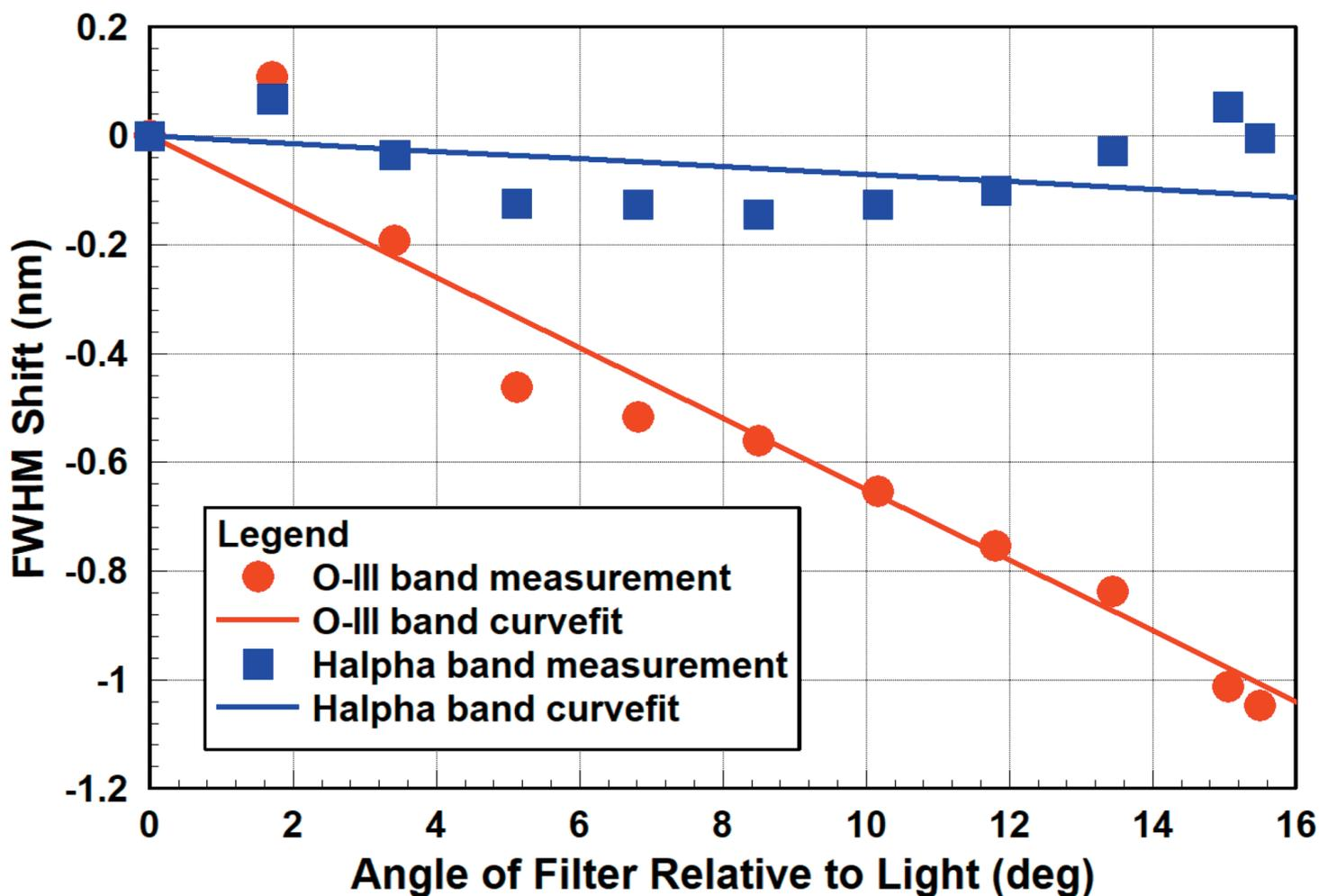
Figure 7 - Measured Radian Triad FWHM Shift vs Angle
