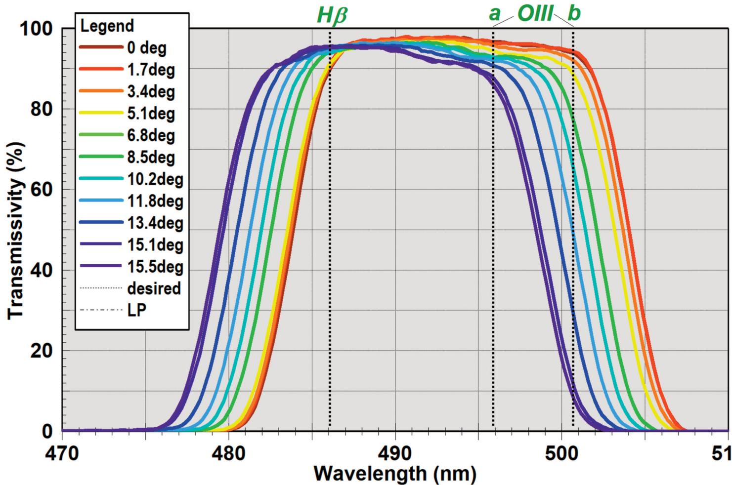
Figure - 4 Measured Radian Triad Spectral Response vs Angle – O-III Pass Band
