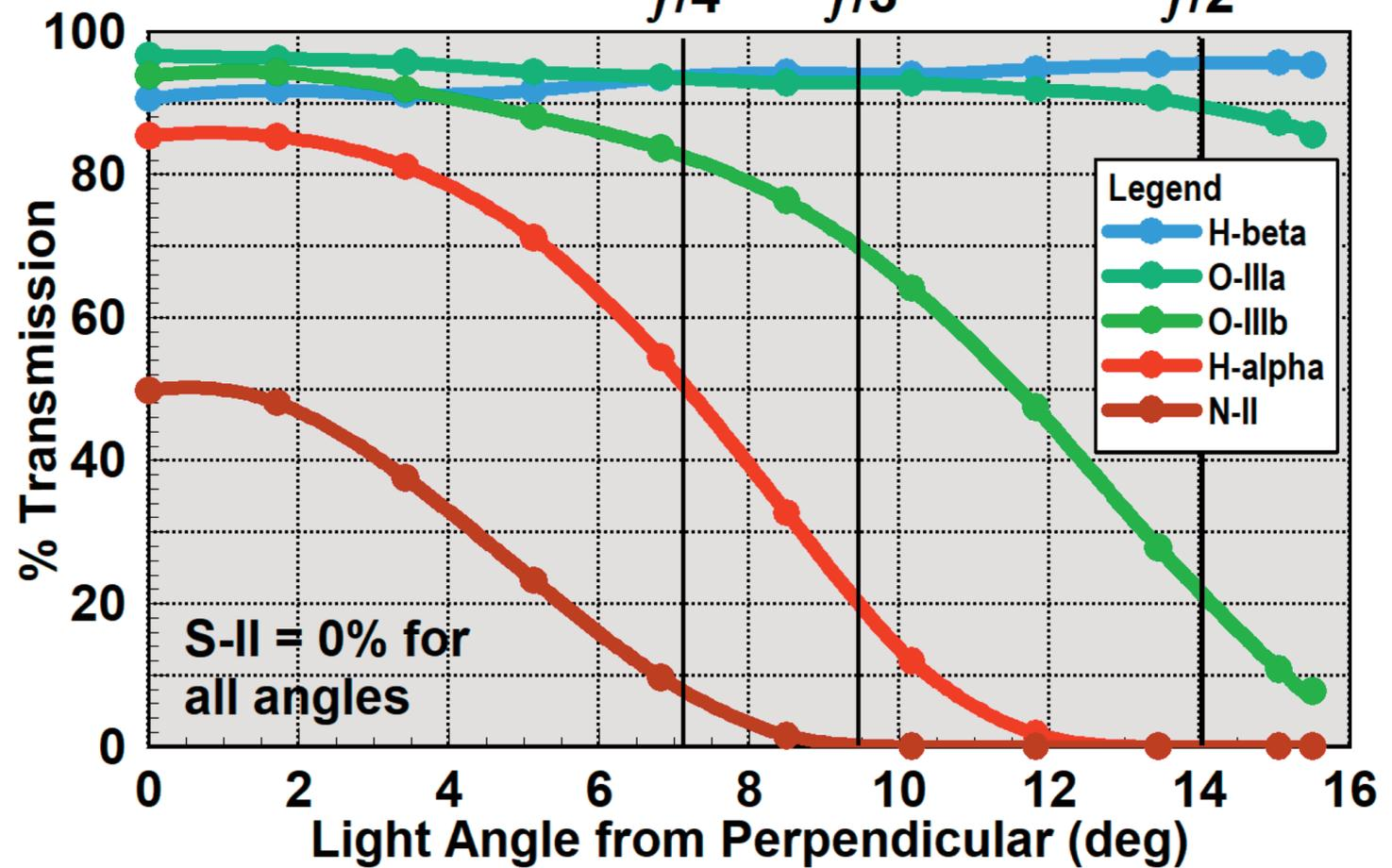
Figure 9 - Measured Radian Triad Nebula Wavelength Transmission vs Angle
