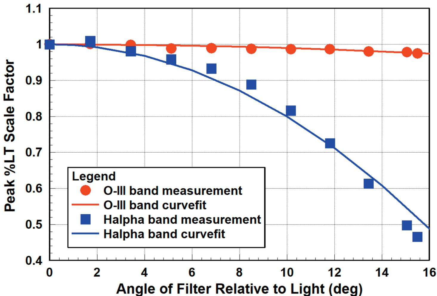
Figure 8 - Measured Radian Triad Peak %LT Scale Factor vs Angle
