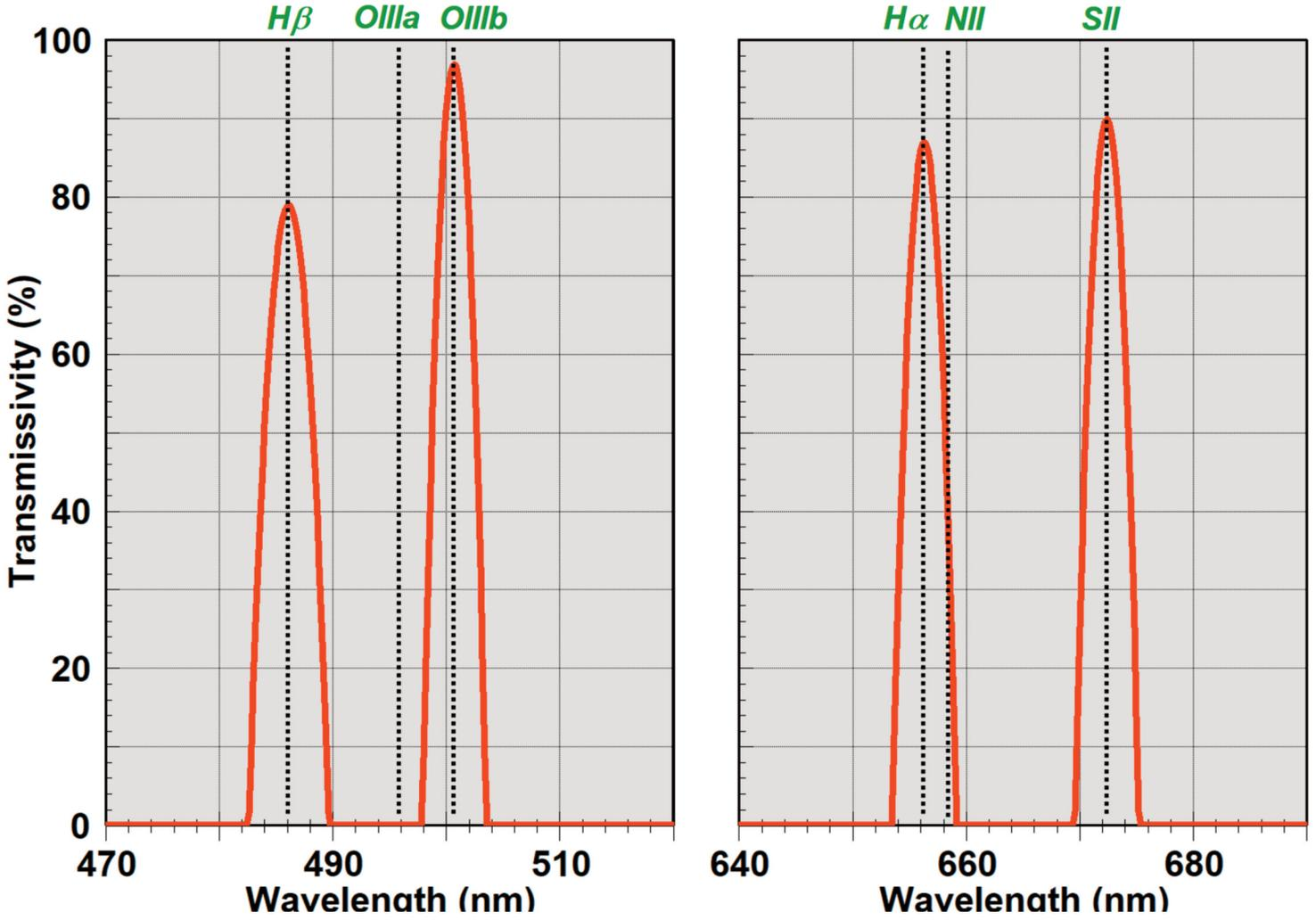
Figure 10 - Theoretical Radian Triad Ultra Spectral Transmissivity
