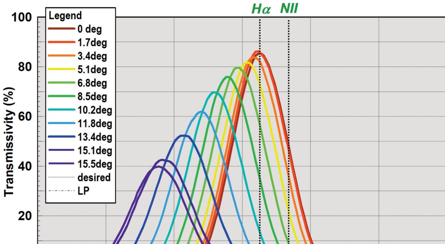
Figure 5 Measured Radian Triad Spectral Response vs Angle – Halpha Pass Band
