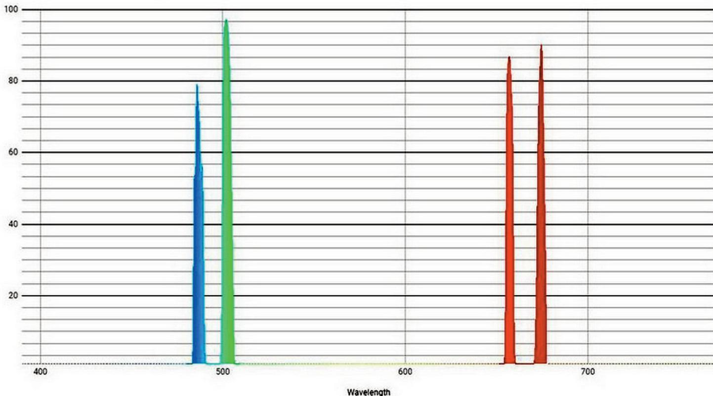
Figure 2 - OPT Radian Triad Ultra Spectral Response (courtesy OPTCorp)
