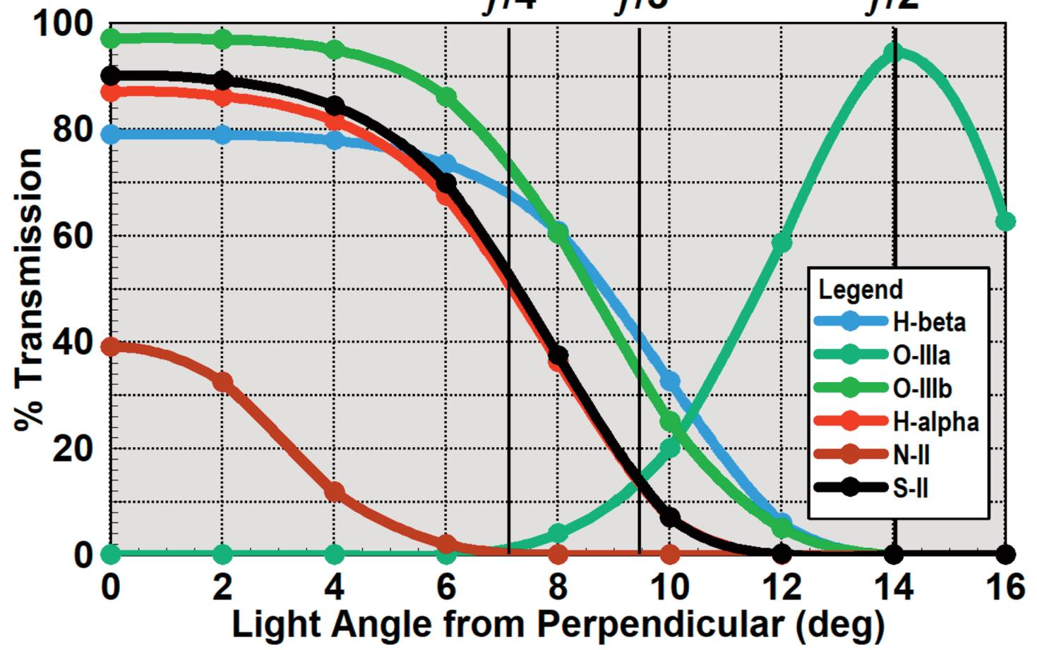
Figure 11 - Theoretical Radian Triad Ultra Nebula Wavelength Transmission vs Angle
