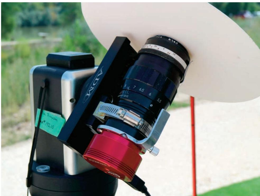
Figure 3 - Eclipse day image of lens, camera, and filters on Cube Pro mount.
