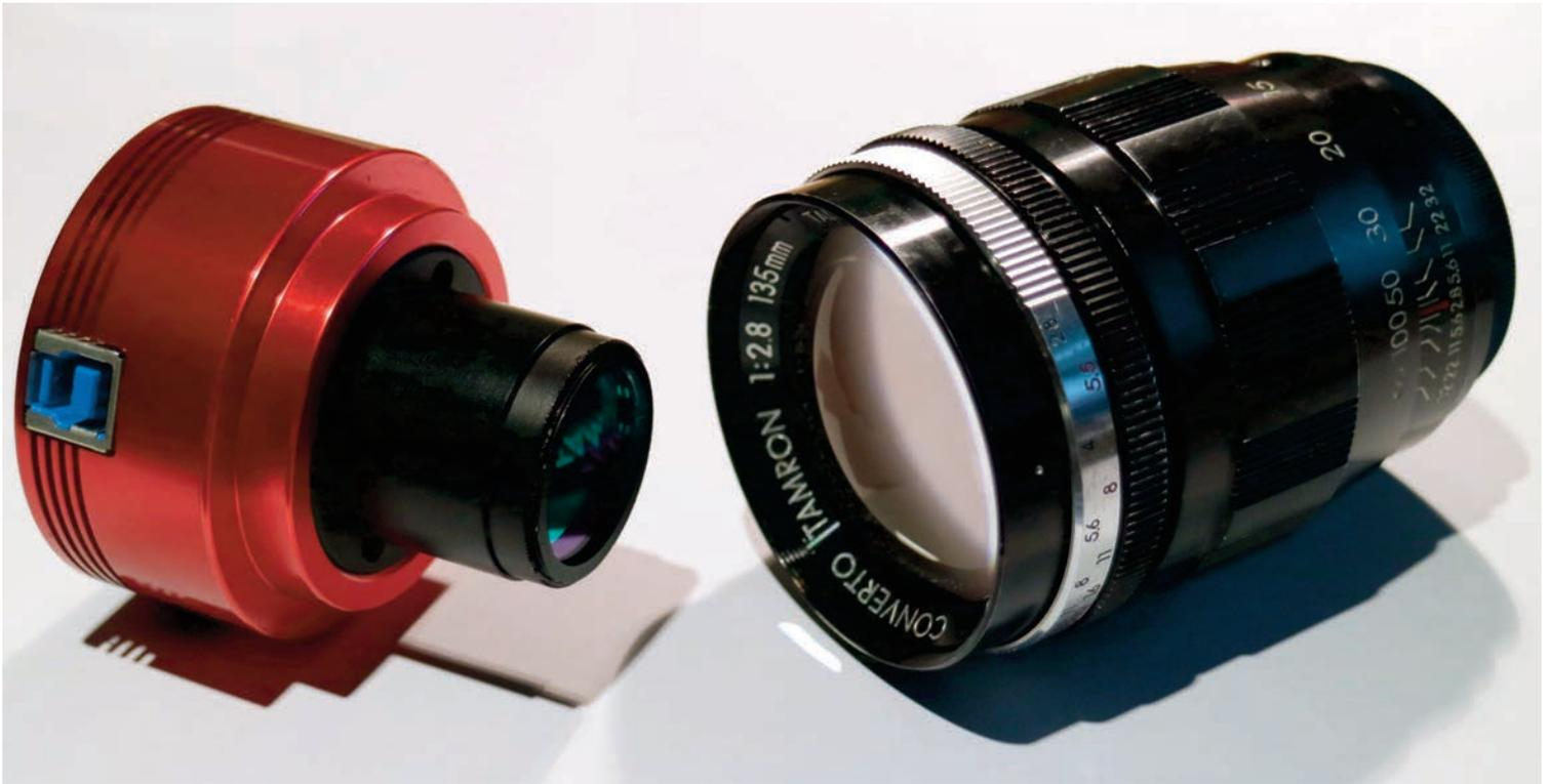
Figure 2 - Image of ASI290 camera and manual 135mm Tamron lens used in imaging setup.
