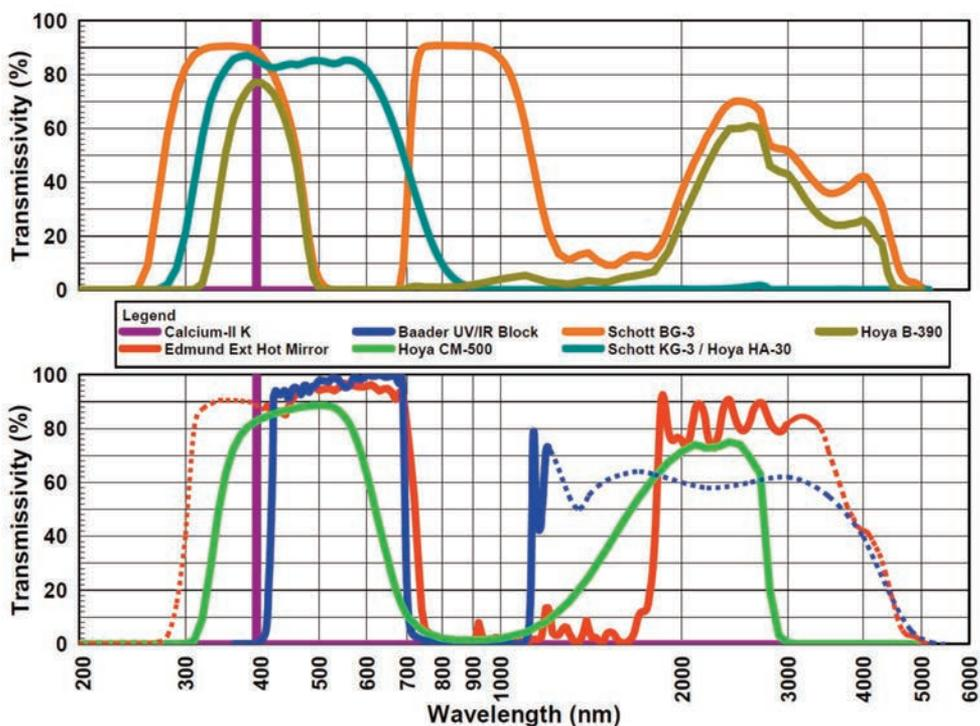
Figure 5: Response curves for the filters used in solar heating tests.
