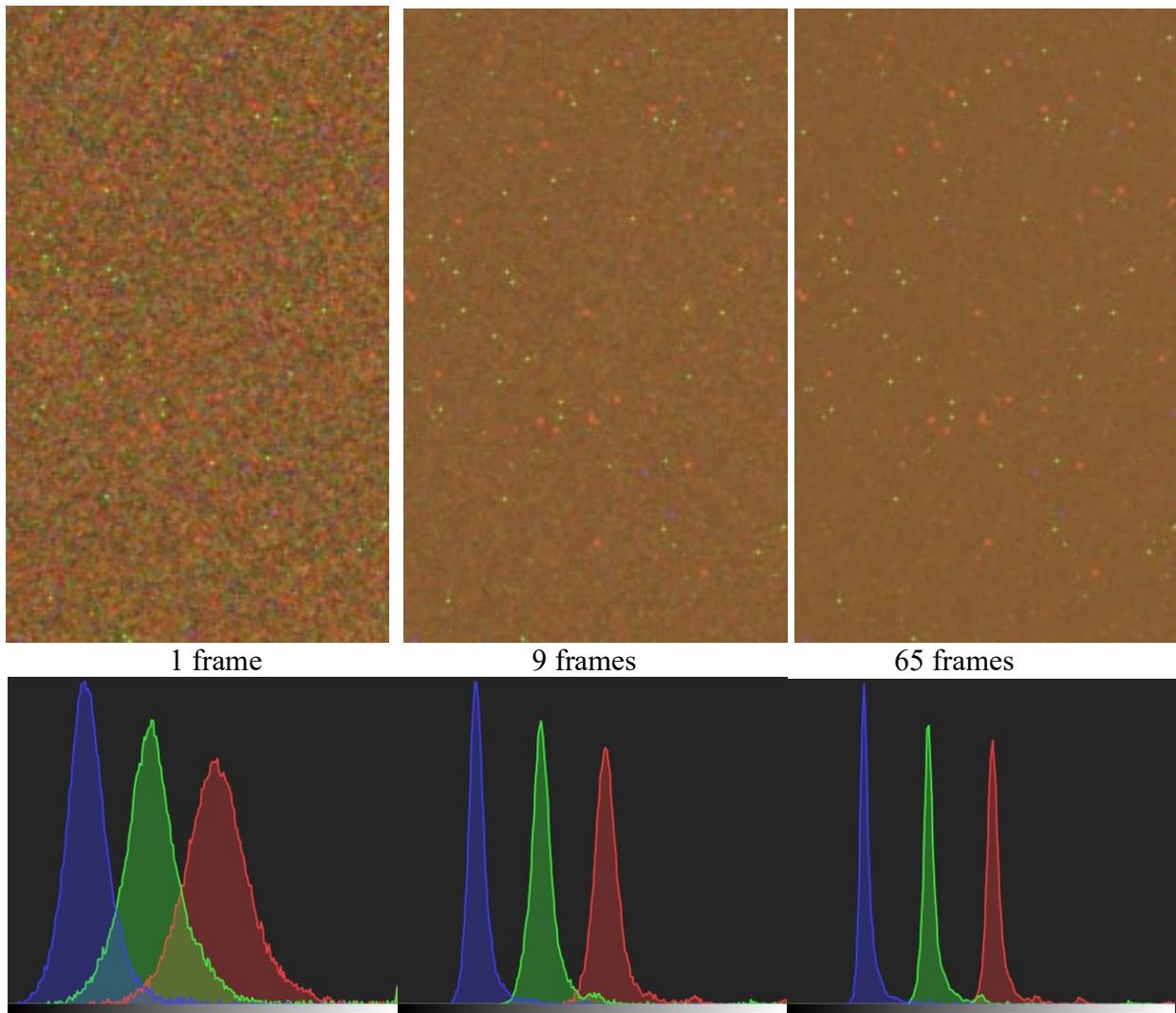
**Figure 3 ASI294MC-Pro Signal Images @ Various # Stacked Frames, no TEC**
