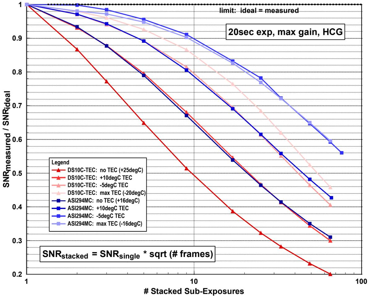
Figure 4  $SNR_{measured}/SNR_{ideal}$  For Both Cameras
