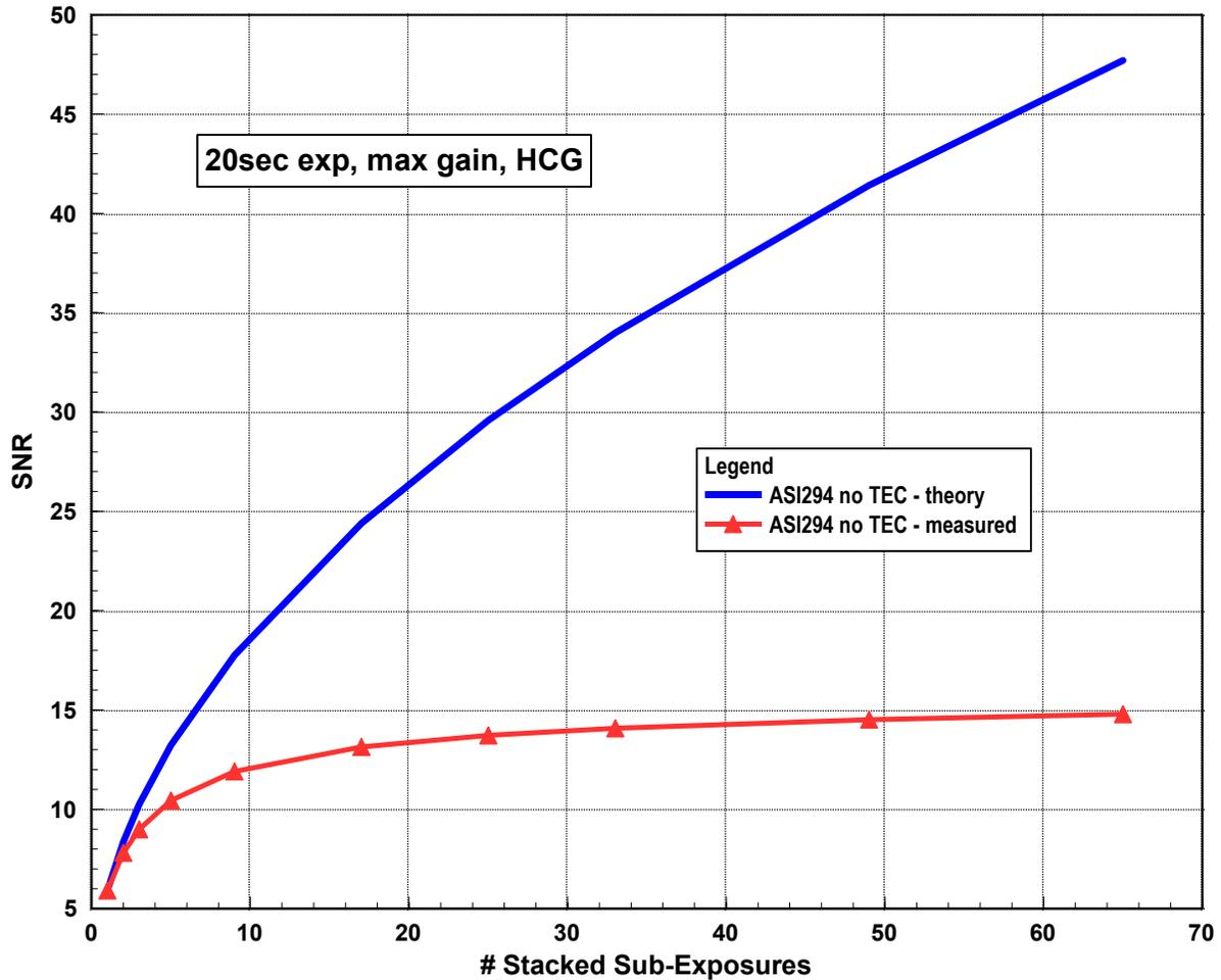
**Figure 2 SNR Measured vs. Theory, ASI294MC Pro - no TEC**
