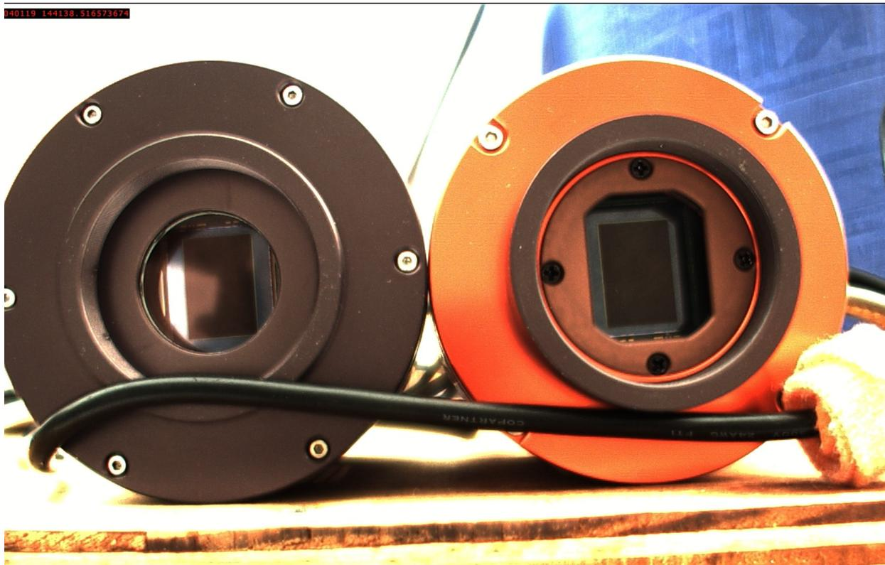
**Figure 1** Image of Cameras During Anti-Fogging Test
