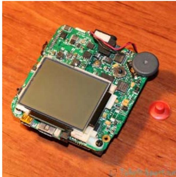
To remove the battery, *gently* separate the PCB located on the top left from the main PCB. To do this, use both thumbs and forefingers, and pinch the PCB on both sides. Rotate your fingers towards the PCB, so that they push against the main chip and separate it from the main chip. (In effect, use your fingers to pry it up, using the main PCB as the fulcrum.)
