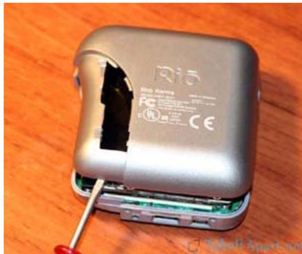
**It is important that the battery is not removed at this point.** Doing so will tear the wires and ruin the Mp3 player.
