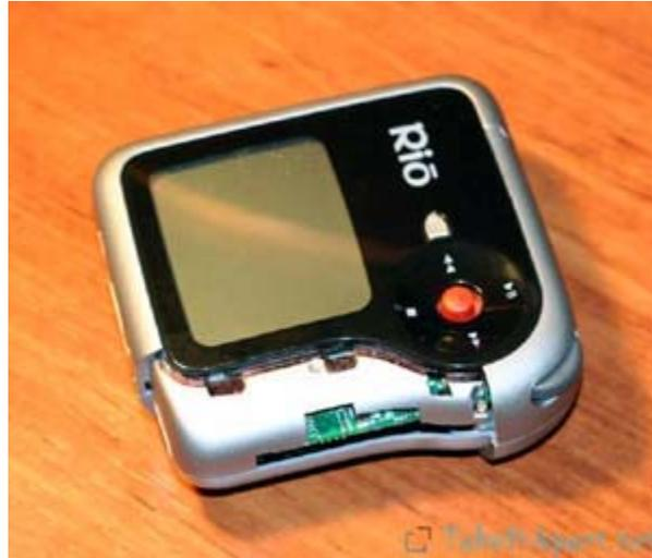
This next step is to be performed very **carefully**. Gently wiggle a small flathead screwdriver or device between the two main halves of the Karma. Be careful not to force it too much, or to push it in too far, as this may cause permanent damage. Continue wiggling the wedge, and slowly sliding it down the seam until the two halves totally separate.
