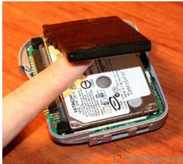
**Do not** remove the two screws holding the hard drive together. Notice that there are now two screws sitting *outside* the perimeter of the hard drive, **Not the screws attached to it!!!**
