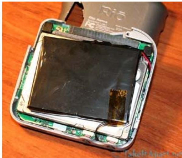
Removing the screws near the edge of the PCB screws will allow the entire PCB-HDD-Battery module to be removed from the case.
