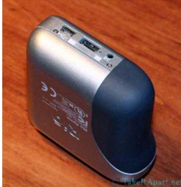
After the screws are removed and stored safely (in a cup or other such vessel), the next step can be performed. Pinch the dark gray thumb rest near the screen and pull out to the right, to remove it from the device.
