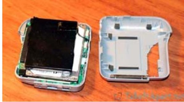
If the battery is lifted *lightly*, you can see the hard drive resting underneath.
